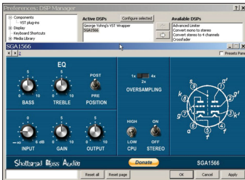
Photo 2: This foobar2000 screenshot shows the George Yohng's VST wrapper and the SGA1566 in the Active DSPs panel. Clicking SGA1566 and then the Configure selected bar displays the plug-in's screen. I used the setup shown here for the measurements.
