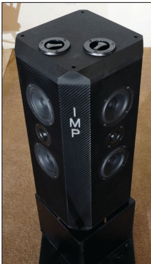
Photo 1: The speakers were built by Dan Neubecker, a consultant for Parts Express, with variable pots for the front panels providing an adjustable radiation pattern.
