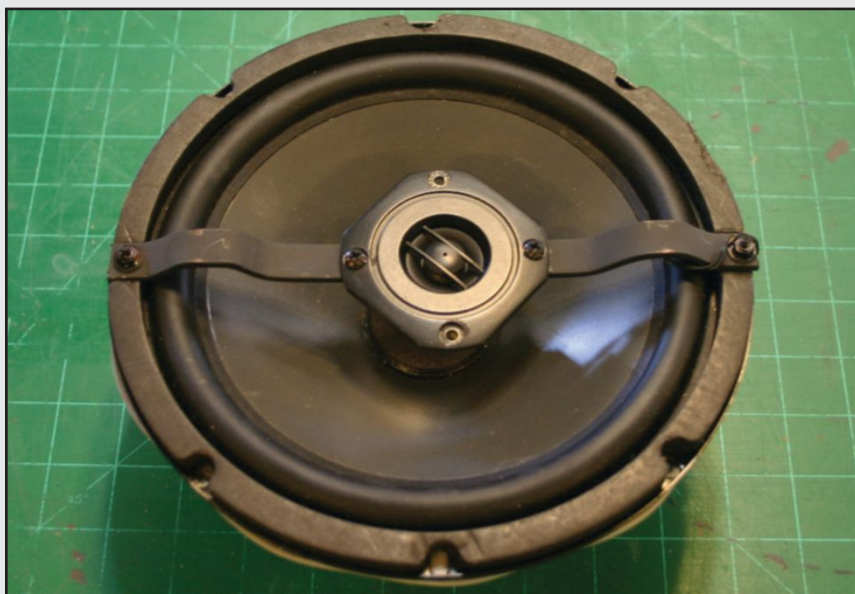
Photo 9: This is another coaxial speaker made from a Goldwood dome tweeter and an Audio Concepts 8" raw driver.
