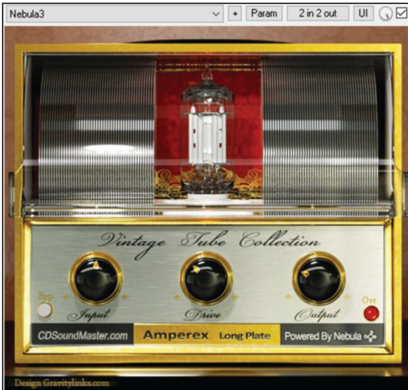
Photo 4: The selected dual triode name, Amperex Long Plate, is displayed bottom center. The Vintage Tube Collection screen is colorful and attractive but the knob’s small size, highlighting, and lack of calibration marking makes set up a chore. However, it works wonderfully. The light colored dot in the lower left corner is the Bypass switch and the red dot, lower right corner, is a clipping indicator.
