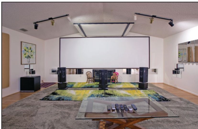
Photo 2: Mirror tiles at all first reflection points enable you to actually see all reflected sources, plus help ensure sharp focus and flat response of those sources. This is a sat/sub system with a Velodyne F-1800 and a center and surround speakers for movies and more audio choices.
