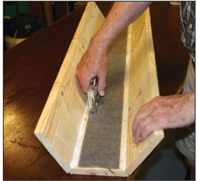
Photo 4: Staple the indoor/outdoor carpet to the inside surfaces.
