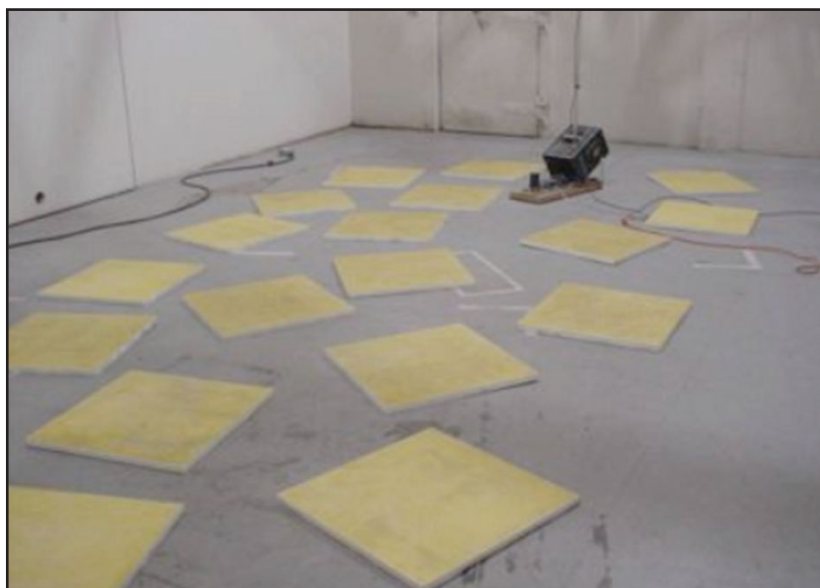
Photo 1: One sample consisted of 2’ x 2’ squares of absorptive material. (Image courtesy of NWAA Labs)
