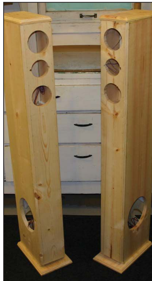
Photo 9: The raw enclosures are ready for sanding and final finish.
