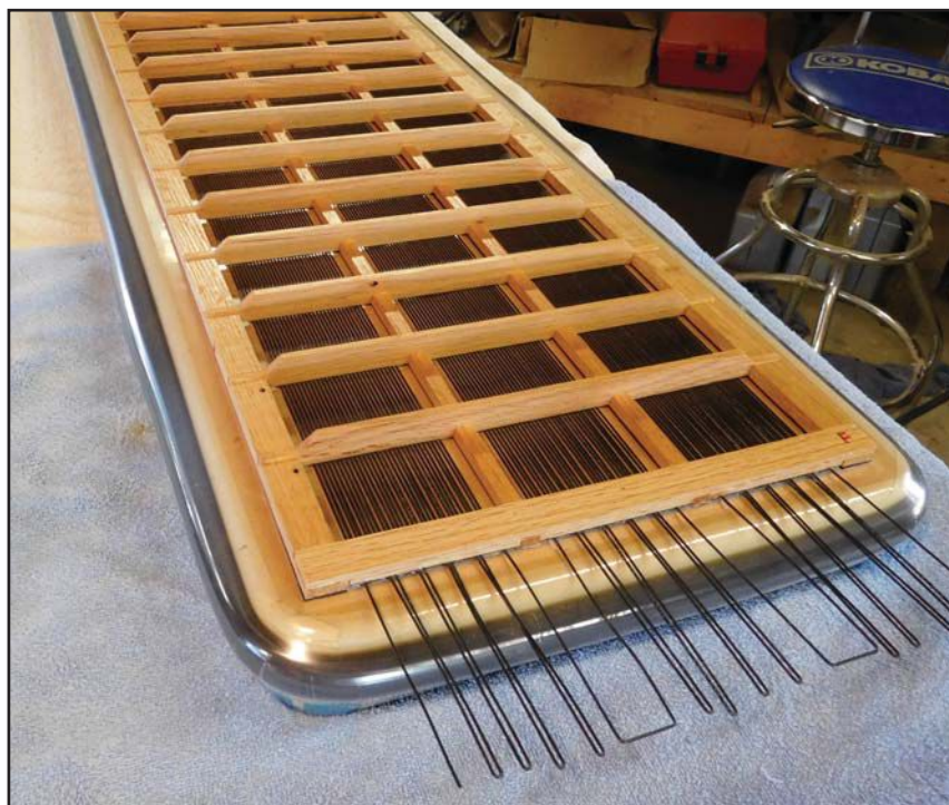
Photo 6: Next I bonded the stator to the diaphragm, on the tensioning jig.
