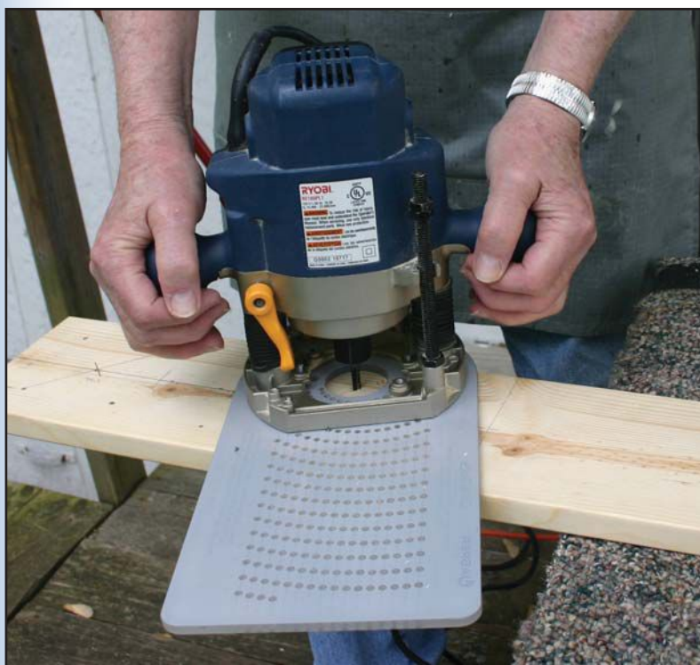
Photo 5: The Jasper circle cutting jig was used to cut all the speakers openings. It enables circles from 2" to 18" to be cut to the necessary increments.
