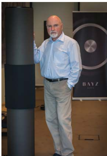
The Bay Radial Speaker is actually a cylindrical membrane surface capable of changing its diameter.
