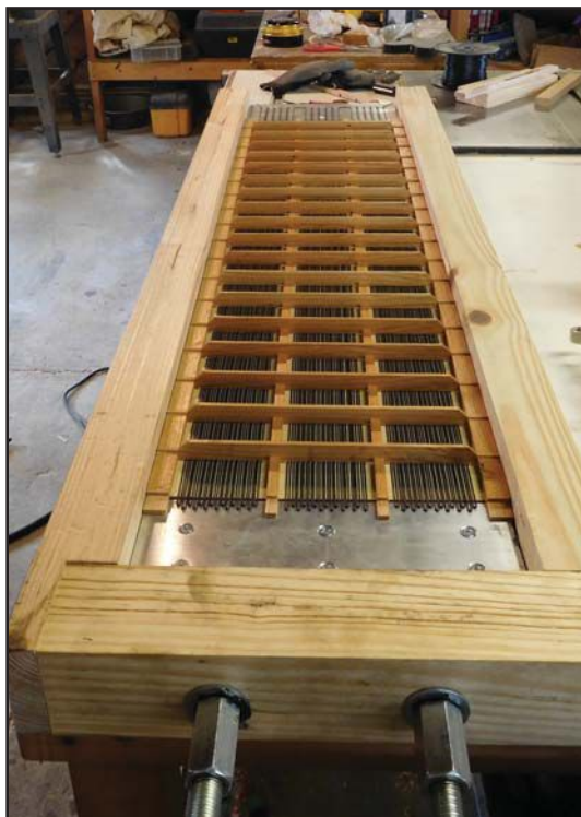
Photo 4: I assembled the stator support lattice over the wires in the stretching jig.
