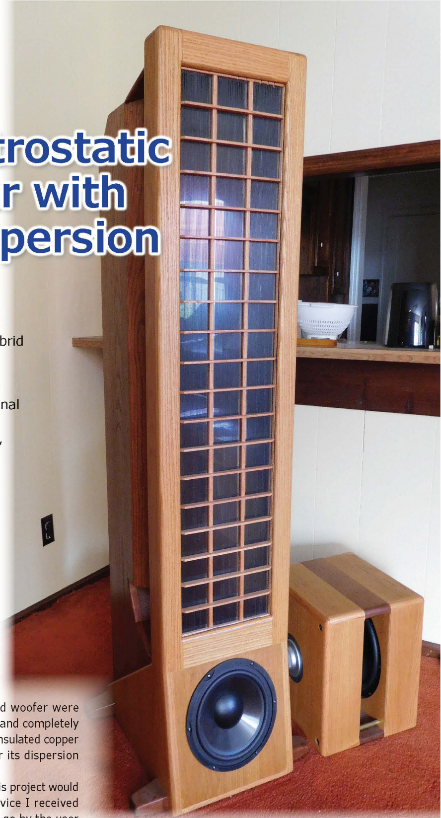
Photo 1: This project is a hybrid ESL with electrically segmented wire stators.
