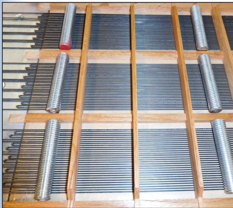
Photo 5: All-thread rods hold the correct wire spacing while you are gluing the oak support lattice onto the wires.
