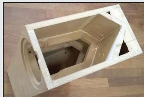
Looking into the lower portion of the Rinjani prototype cabinet. This photo also reveals internal bracing and the inner wedge-shaped rear wall, behind the midwoofers only, that significantly reduces the reflected sound wave.
