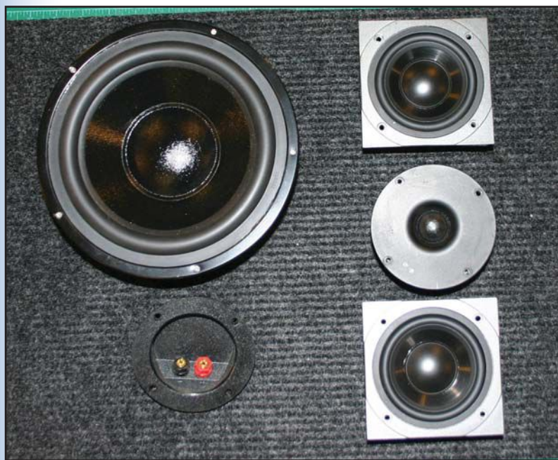
Photo 2: The drivers and terminal cup used in the Thinman include the Dayton 8" woofer, two 4" midrange units, and a dome tweeter.
