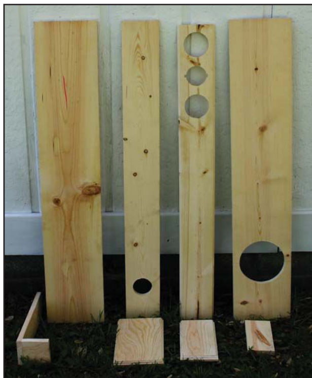
Photo 3: The precut lumber required to construct one enclosure is shown.
