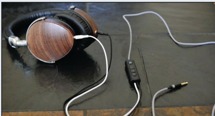
Photo 1: Uniquely combining science and design, Even's H1 Headphones feature a patented EarPrint technology with an on-board hearing test and real-time frequency compensation.
