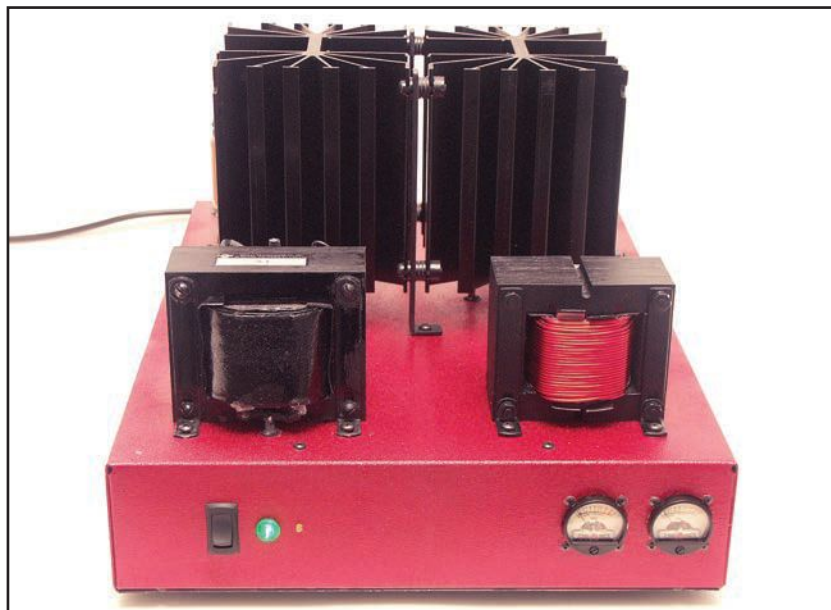
Photo 2: When we complete the project, our Cherry Bomb VFET SET preamplifier should look like this. Here is a front view with the VU meters illuminated.
