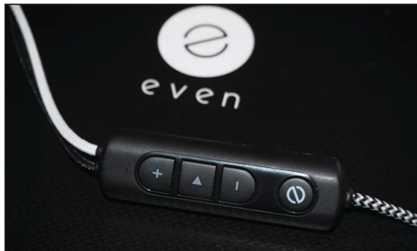
Photo 3: The Even EarPrint’s electronics fit into an earphone remote control and include a dedicated button to toggle the compensation on and off.
