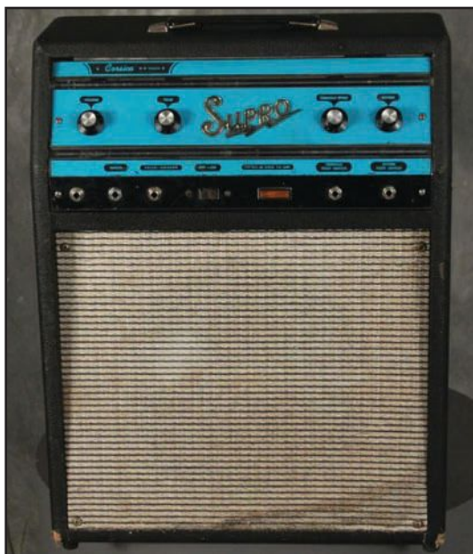
Photo 2: The Supro S6622 offered reverb, tremolo, more power, and a better sound than the low-priced AC/DC-supply amplifiers.
