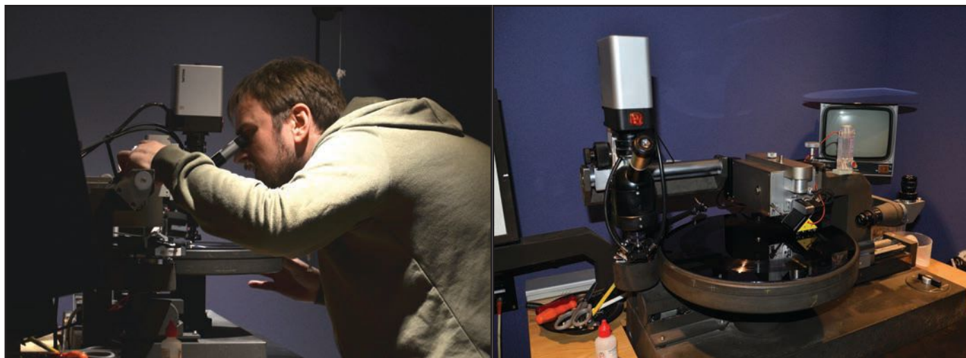
Cutting engineer John Webber uses a microscope to check the Neumann VMS 80 cutting lathe. At right is the lathe making the LP mastering.
