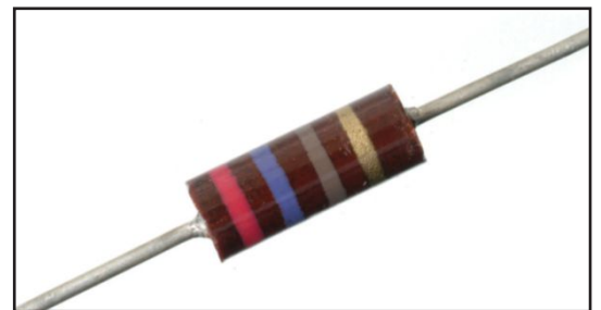
Photo 2: A carbon composition resistor can be recognized by its near-perfect cylindrical shape.
