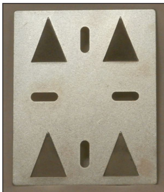
Photo 2: The stamped metal impaler plates measure about 3" x 4". Attach them to your wall with the points facing up. I found using a large screwdriver or small pry bar to bend the points closer to 45° made it easier to attach the panels. Place a plate against the wall, mark the hole locations, and drill two 0.25" holes (the drill bit is provided), insert the plastic expansion plugs and affix the plate with two of the provided screws.
