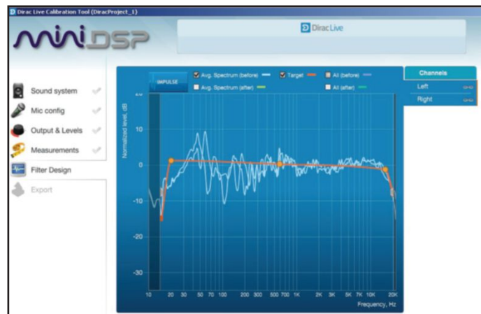
Photo 6: When all nine measurements are completed, this screen displays the averaged left and right responses with a default target curve. Their target has more tilt than I like so I grab the orange dot control points and flatten it some. You can add additional control points by clicking the orange target curve.
