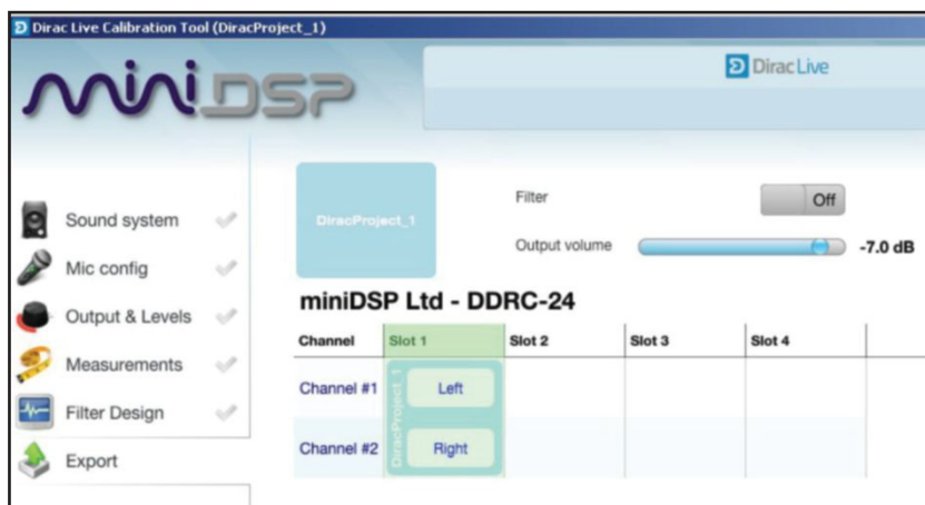
Photo 8: Drag the blue square with the project name into Slot 1 to program the DDRC-24. I captured this screen after the programming so Slot 1 displays Left and Right as the channel names. Remember to turn the filter On, and to set the Output volume before exiting.
