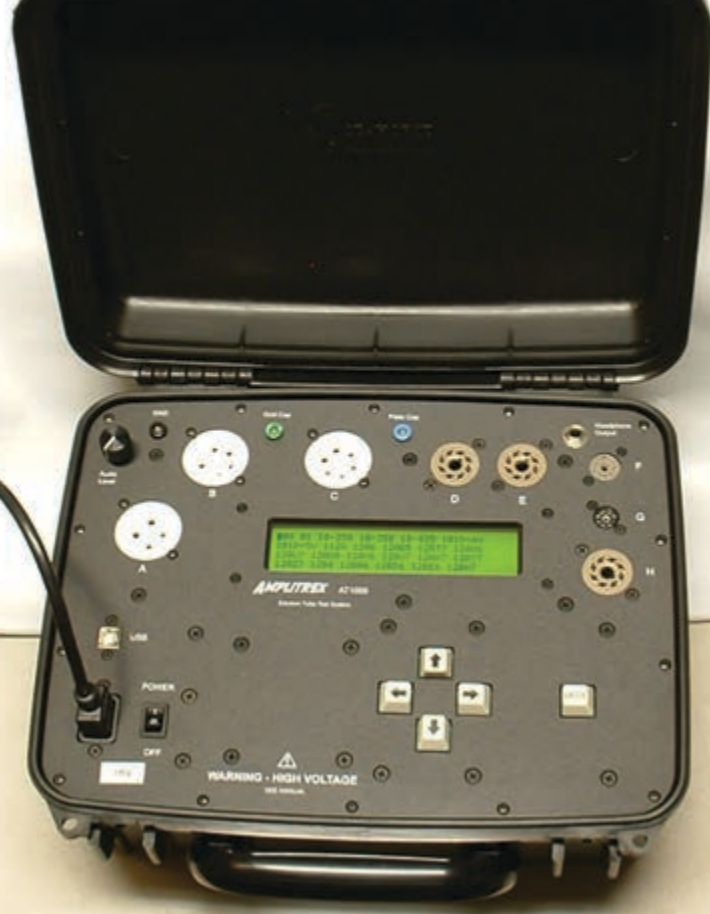
Photo 1: The AT1000 provides comprehensive test functions for electron tubes.
