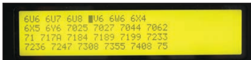
Photo 2: The user selects the tube type to be tested in this screen. (Photo courtesy of Amplitrex)
