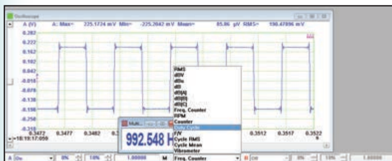
Figure 4: The Multimeter is displayed overlaying the Oscilloscope screen, in this case showing the frequency of the square wave. The menu for other Multimeter options is also shown.
