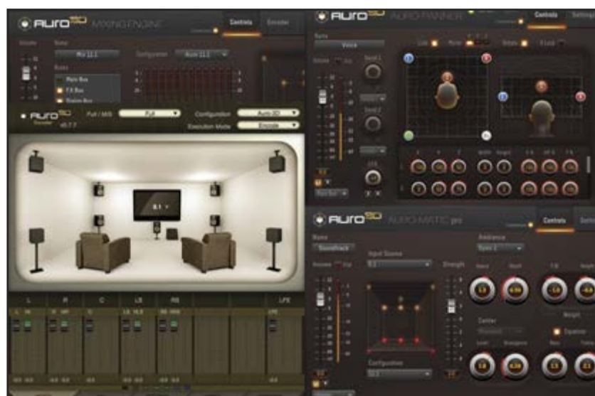
Photo 2: The Auro-3D Creative Tool Suite enables users to add immersive 3-D sound to any existing production workflow, while making the 3-D content available through a standard PCM single-file distribution. It is played back via existing standards such as DCP in digital cinema or via Blu-Ray for the home theater to reproduce in each channel high-resolution audio (HRA) to experience the sound as it was intended by the creators.
