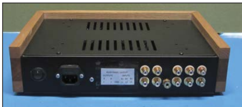
Photo 3: The rear view of the deluxe version shows the inputs and the outputs.
