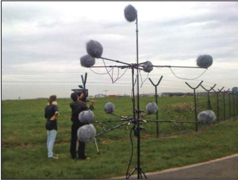
Photo 3: An Auro-3D crew recording in an outdoor setting. No information is included with the photo, but from the setting and microphone arrangement I suspect an aircraft flyover. The top, height, and lower recording levels are clearly shown.
