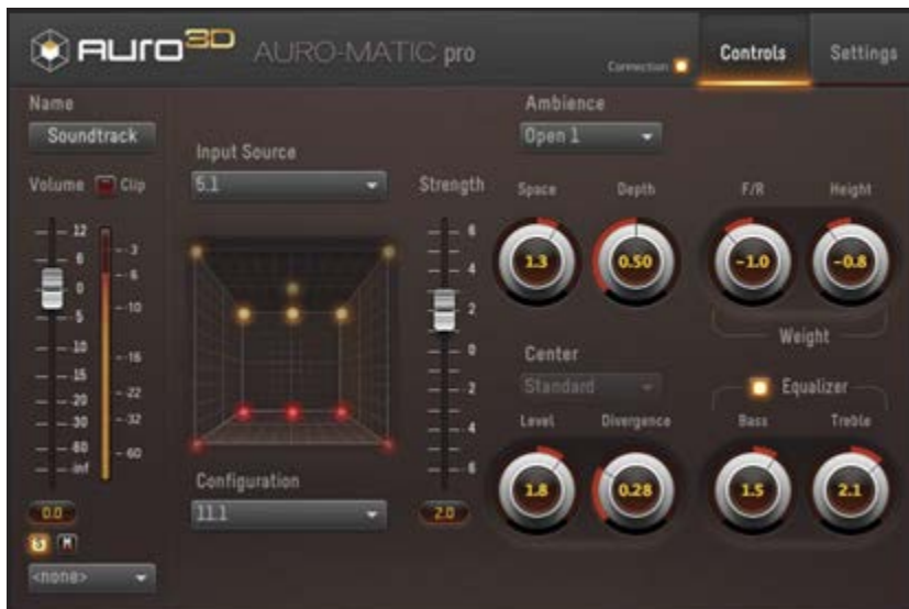
Photo 4: The Auro-Matic Pro 3D main screen lets you select the input and the output formats and variables including spatial size, the balance between front and rear, and the balance between the lower and height channels. Complete details are in the user guide.
