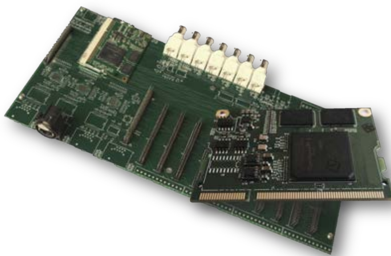
Coveloz’ AES67/Ravenna and Ethernet AVB audio networking and processing FPGA Development Kit offers a robust design platform built around the Altera Cyclone V System-on-Chip (SoC) FPGA. This kit is also host to the BACH-SOC firmware that provides FPGA and Linux firmware, enabling customers to quickly build AVnu-certified and AES67-capable products.
