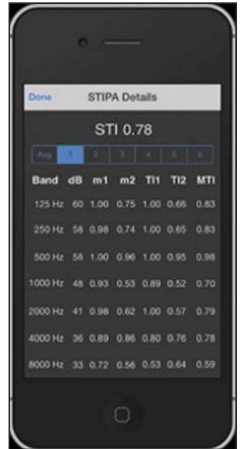
Photo 16: The octave-band details of the Speech Transmission Index (STI) measurement can be viewed once the measurement is complete.
