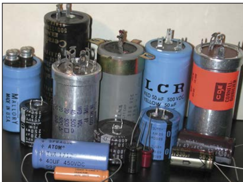
Photo 1: Bad capacitors or nonlinear distortions generated by capacitors are a common source of problems.
