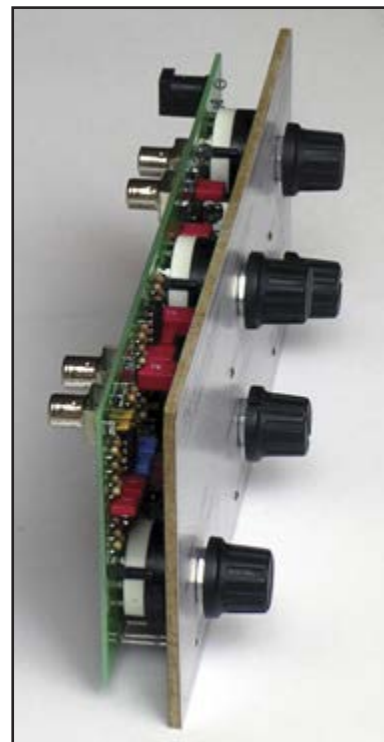
Photo 6: The LEDs and the rotary potentiometer leads are soldered after the panel is mounted because the lead length is determined by the panel-to-board spacing.
