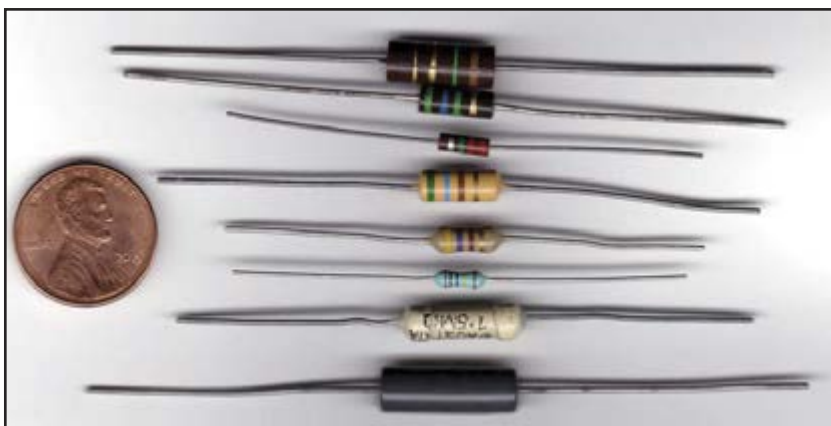
Photo 1: Resistors of different technologies have different noise performance: (from top) 1 W carbon-comp, 0.5 W carbon comp, 0.5 W carbon film, 0.25 W carbon-comp, 0.5 W carbon film (different manufacturer), 0.125 W metal film, 1 W wirewound, and 2 W wirewound.
