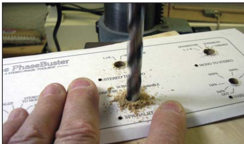
Photo 4: The PhaseBuster's front panel was made from 1/8" Masonite.
