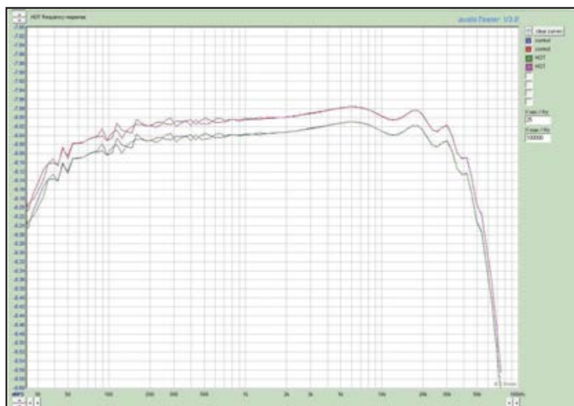
Figure 8: This is the frequency response across the simulated headphone load with and without the enhancement device. Note the expanded scale. The mismatch of 0.02 dB between right and left channel is well within the sound card specification and is negligible.
