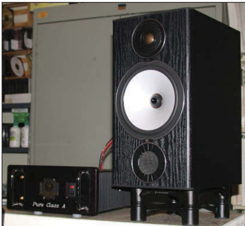
Photo 6: For the listening tests, I mounted a Monitor Audio Bronze BX2 loudspeaker on an IsoAcoustics Aperta speaker stand. Monarchy Audio's SM-70 power amplifier, operating as a fully-balanced monoblock, is seen on the left.
