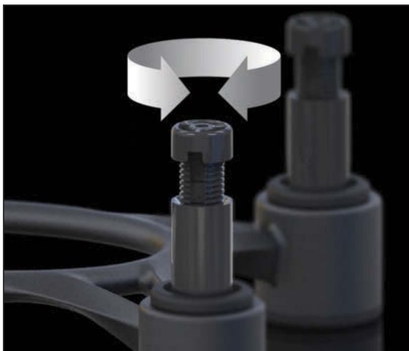
Photo 3: Threaded inserts in two of the aluminum support rods enable a tilt adjustment of up to 6.5°. By rotating the stand 180°, the speaker can be tilted backward or forward. A red mark on the threaded inserts appears when the maximum tilt angle has been exceeded. (Photo courtesy of IsoAcoustics)
