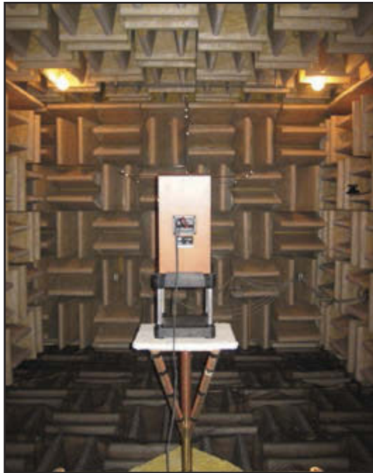
Photo 4: A loudspeaker is shown mounted on an IsoAcoustics isolator, which was tested with a laser vibrometer in an anechoic chamber at the Canadian National Research Council in Ottawa, Canada. (Photo courtesy of IsoAcoustics)
