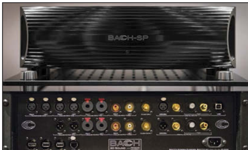
Photo 2: The BACCH-SP processor's front panel hides the filter selection buttons and the controls to program a custom filter matching the listener's head and room description.
