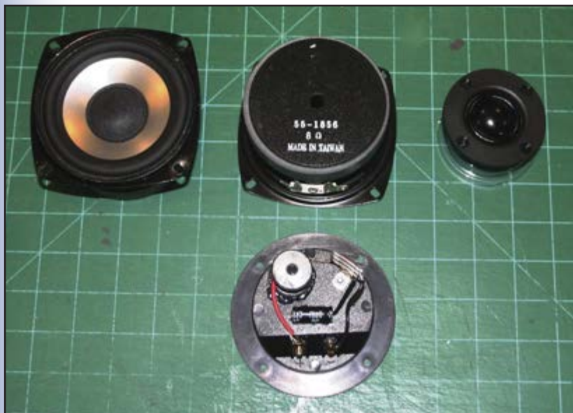
Photo 5: The drivers used in the system are shown with the terminal cup. Note the crossover components mounted on the cup.
