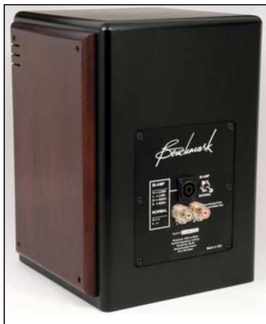
Photo 4: The rear view of the SMS1 loudspeaker shows that each unit has a four-pole Neutrik NL4 SpeakOn connector and a pair of high-quality, gold-plated binding posts. Passive bi-amping is possible via the SpeakOn connector. (Photo courtesy of Benchmark Media Systems, Inc.)
