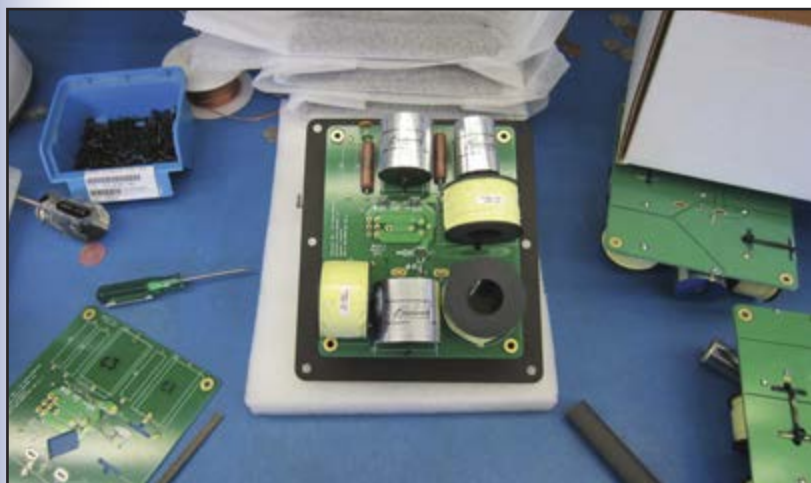
Photo 5: Each crossover board for the SMS1 loudspeaker is hand assembled, using premium-quality parts. ClarityCap custom manufactures capacitors to the exact values Benchmark needs. Custom-wound Renco air-core inductors are oriented to avoid magnetic interactions. Close tolerances are maintained in the crossover components to ensure unit-to-unit consistency.
