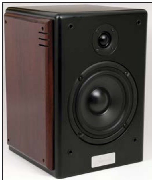
Photo 3: The SMS1, shown in a front view, is an acoustic suspension design using a proprietary 170-mm long excursion woofer and a 25-mm soft-dome tweeter. (Photo courtesy of Benchmark Media Systems, Inc.)
