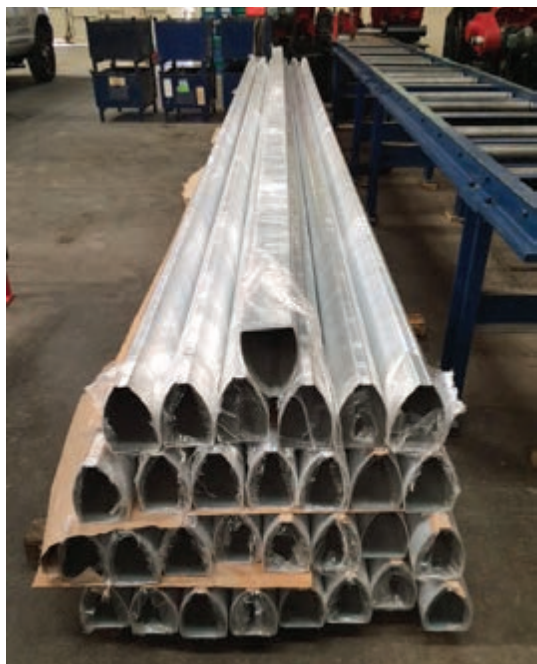
Folded aluminum profiles are used for the speaker cabinet.
