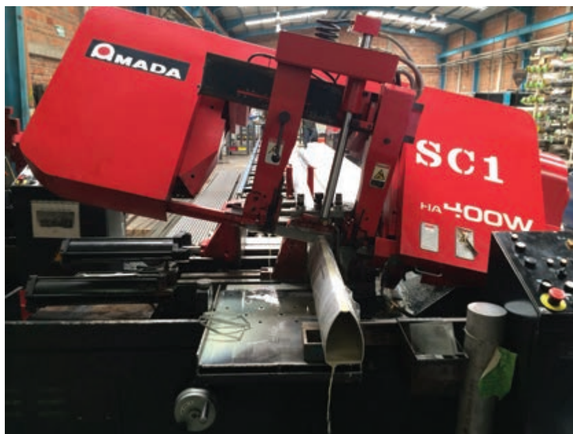
The aluminum profiles are being cut to size during the production process.
