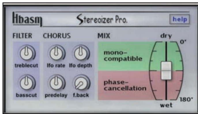
Photo 1: The Stereoizer Pro licensed version activates all the controls and shows the setting number while the control is being adjusted.
