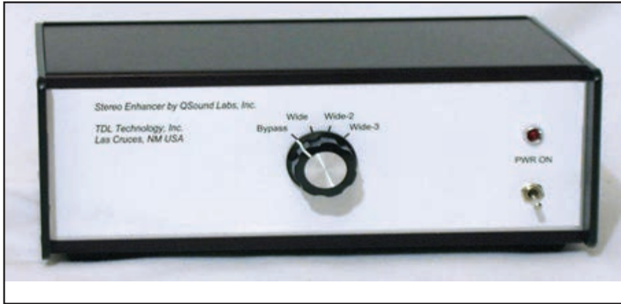
Photo 4: The front panel of the author's demo stereo enhancer, using a QSound QX2130S IC, is shown here. The stereo input and output connectors and the 24 VDC power supply connector are on the rear panel.
