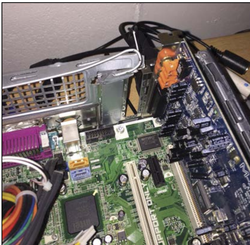
Photo 1: It took some surgery to fit a PCI sound card into a low-level computer! I had to add a few additional components to use a normal-sized PCI card with my low-profile computer.
