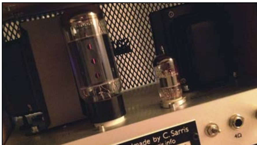
Photo 8: All the tube sockets were made of high-quality porcelain.
