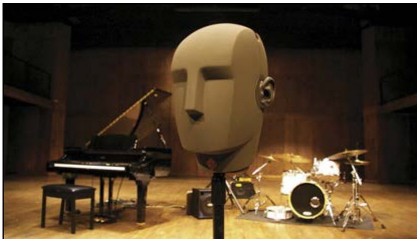
Photo 2: The Kall binaural transducer simulates human hearing. The head has a special microphone built into each ear canal. (Photo courtesy of Kall Binaural Audio)
