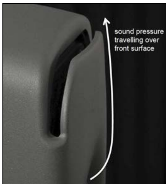
Figure 4: Acoustically concealed woofers radiate low frequency through acoustically optimized openings in the ends of the front baffle. This enables the whole front baffle to be used as a waveguide.
