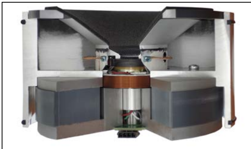
Figure 3: The minimum diffraction coaxial (MDC) design—a 130 mm (5") coaxial driver with midrange and a 19 mm (0.75") tweeter eliminates all diffraction sources, using an acoustically optimized seating of the tweeter and a smooth acoustically continuous surface from the tweeter outward. This design enables good blending to the directivity control waveguide.
