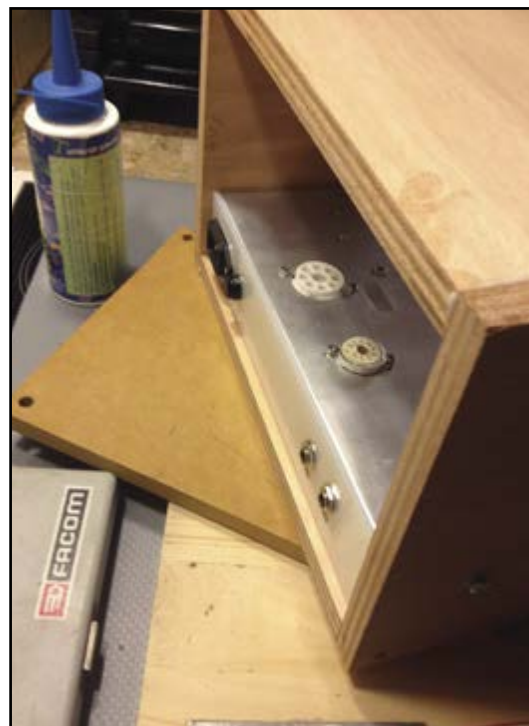
Photo 4: I used a filtered IEC power input connector for the AC input in the power supply.
