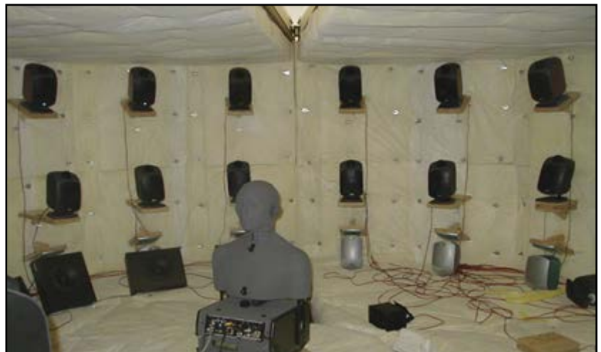
Photo 4: The many loudspeakers grouped around a HRTF head, enable us to convert an array of sound sources to a two-channel binaural output. (Photo courtesy of NIRO Surround Sound Systems, www.niro1.com )
