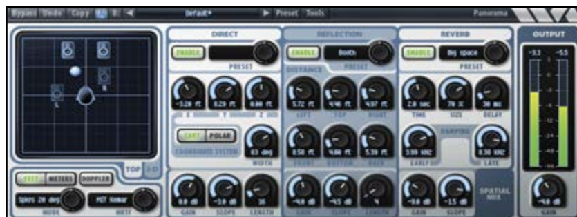
Photo 5: The 24 control knobs on the Panorama plug-in are not easy to adjust for a pleasing result. The manual explains each knob group, but the user is left to experiment.
