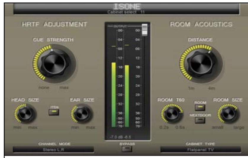
Photo 6: This screenshot of the original Isonne Pro plug-in is functionally similar to the updated ToneBooster's version with areas for HRTF Adjustment and Room Acoustics setup.
