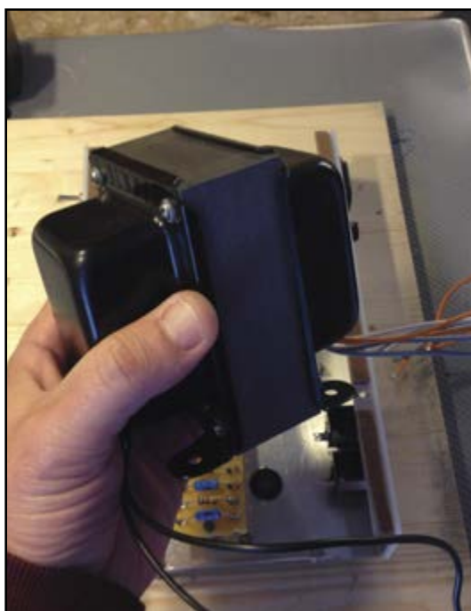
Photo 4: I used a filtered IEC power input connector for the AC input in the power supply.
