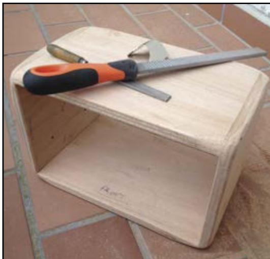
Photo 5: The wood casing is made from handcrafted 16-mm thick birch plywood.
