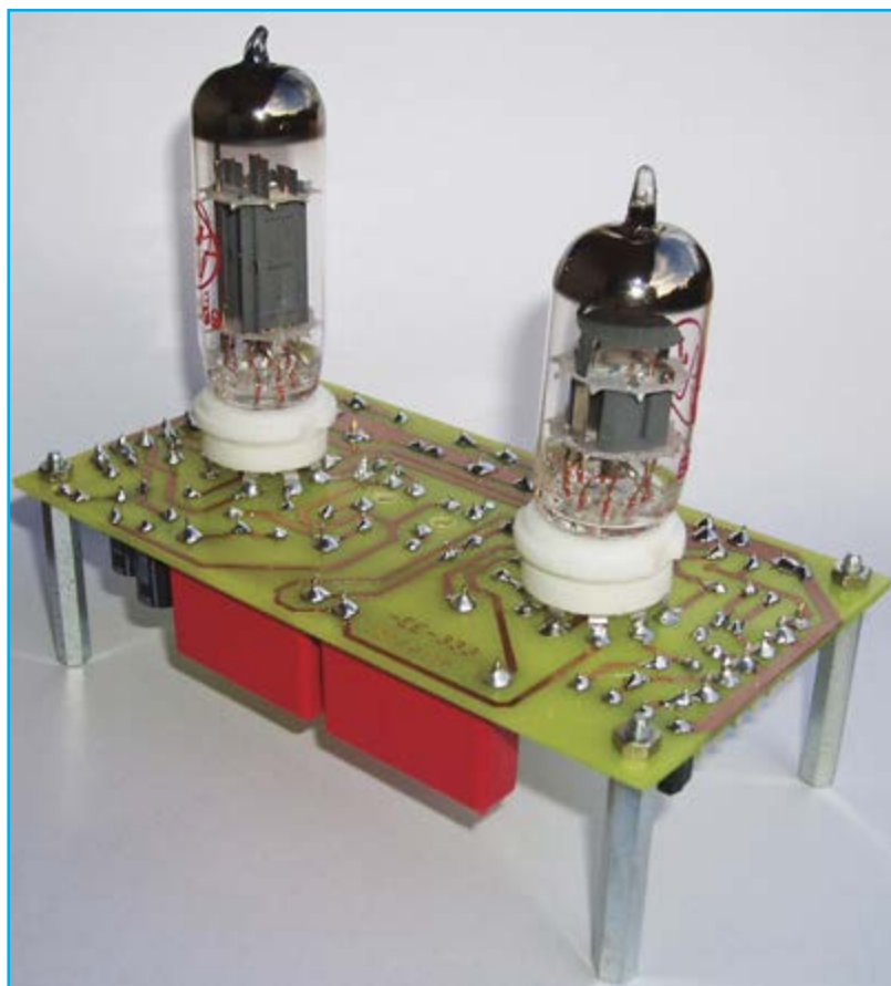
Photo 2: The tube sockets can be mounted so they stand out from the chassis.
