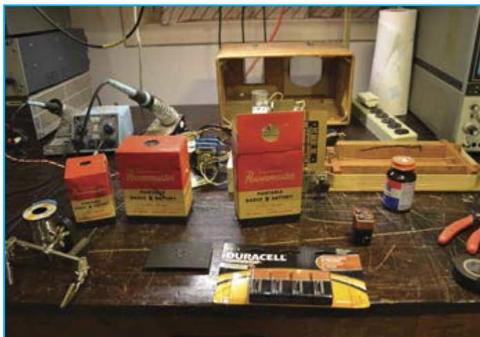
Photo 5: Vintage battery packs supply 90 V across two type-B batteries in series and 1.5 V from one type-A battery. These battery packs can be re-stuffed with modern conventional batteries. In this case, use five 9-V batteries in series to replace one type-B battery and only one size C cell to replace the A battery.
