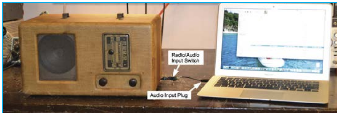
Photo 4: The Sentinel pre-war battery radio has an external audio input that can be connected to a laptop.
