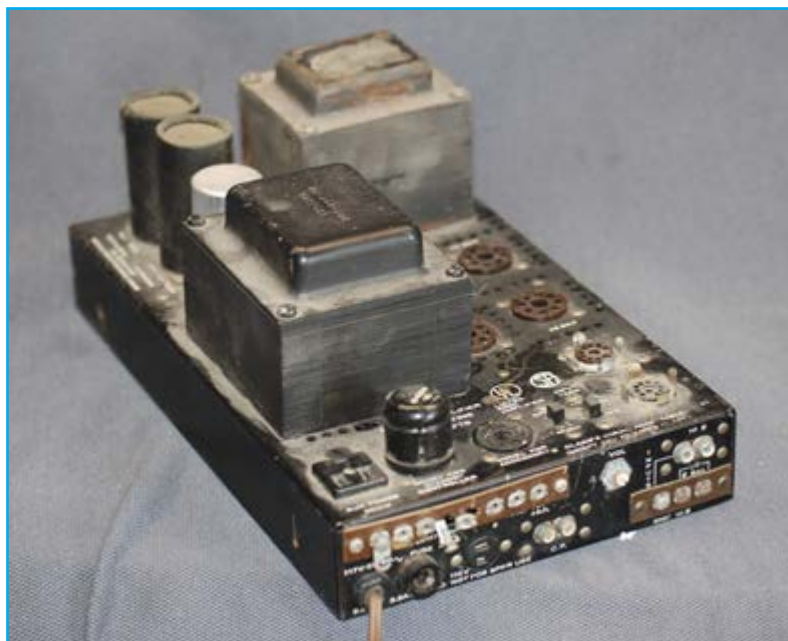
Photo 1: This is the stock Bogen MO100A amplifier as found.
