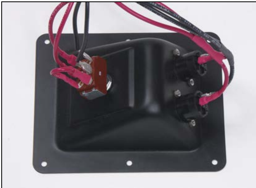
Photo 2: The rear view of the input dish shows the connectors, the switch, and the wiring.
