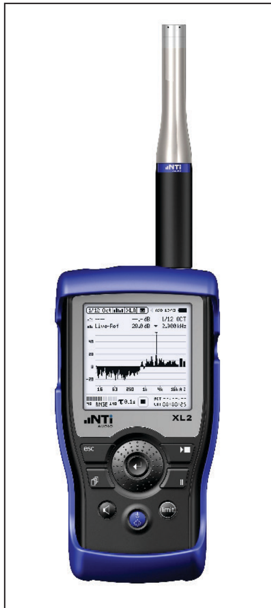
Photo 8: The XL2 is an advanced acoustic analyzer. (Photo courtesy of NTi Audio)
