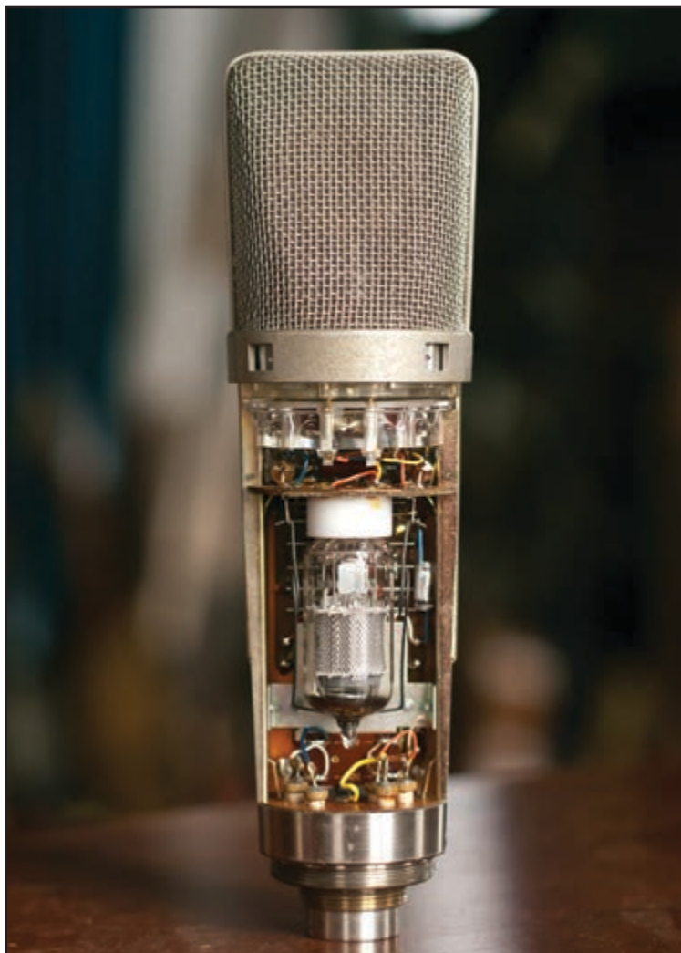
Photo 5: The U 67's interior view shows its construction with an EF 86 pentode. (Photo sourced from Jonathan Low - http://heyjonlow.com/tube-talk )
