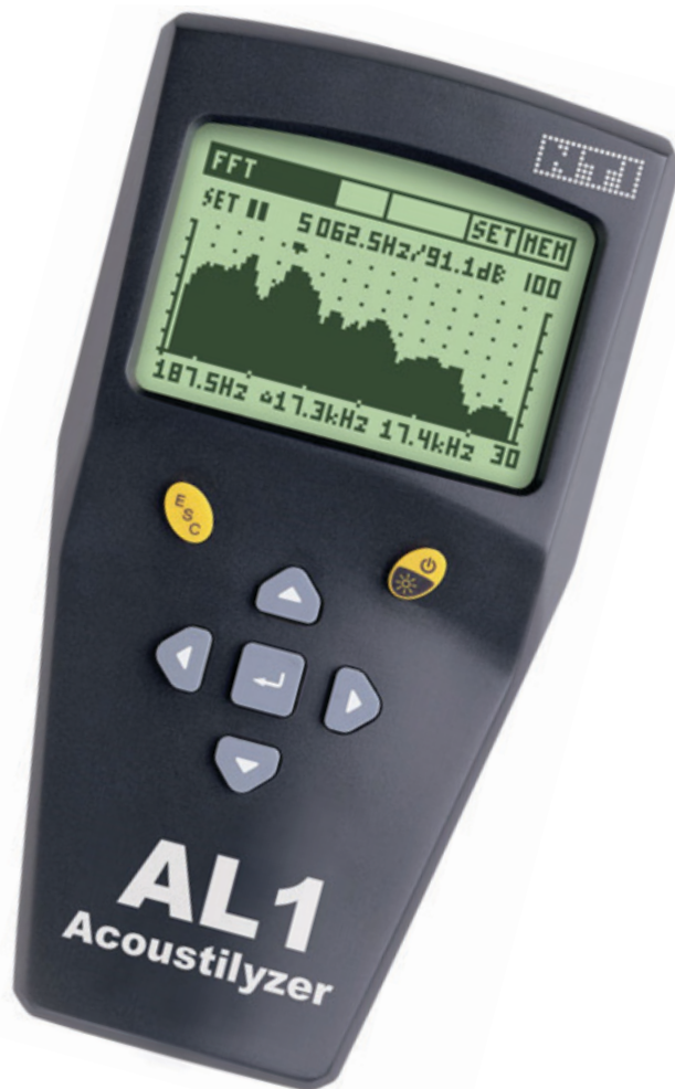
Photo 1: The NTi AL1 is a complete handheld acoustical measuring instrument. (Photo courtesy of NTi Audio)
