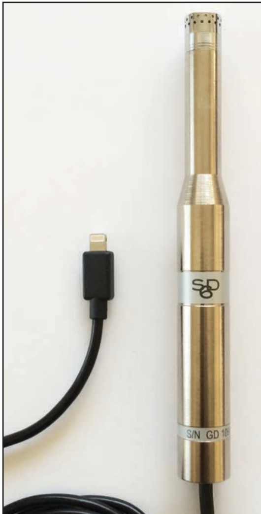
Photo 4: The Studio Six Digital iPrecision microphone is the only ANSI Type 1-certified microphone that is also an iOS direct-connect Lightning accessory. (Photo courtesy of Studio Six Digital)
