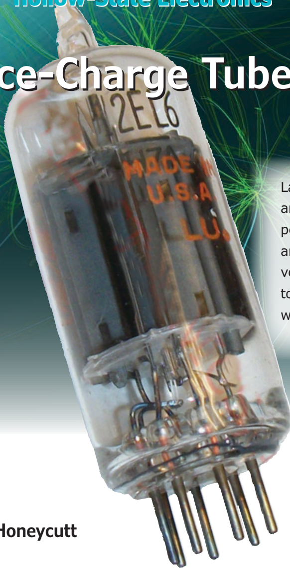
Photo 1: Many of the low-voltage tubes are housed in 7-pin miniature packages.
