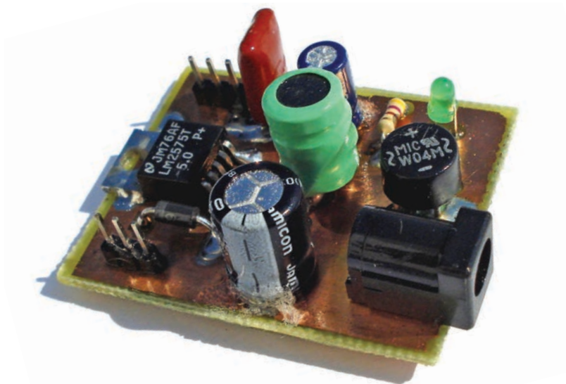
Photo 6: The small power supply unit (PSU) is used to power the volume unit (VU) meter.
