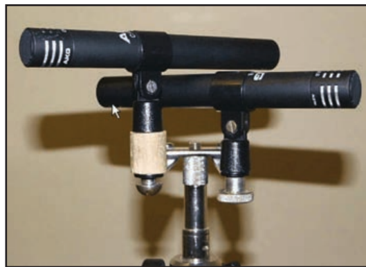
Photo 2: The ORTF microphone arrangement uses an "over-under" pattern on a single tripod.
