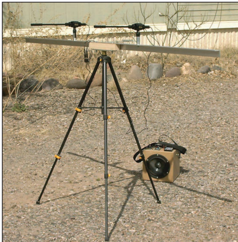
Photo 1: This setup for stereo recording uses two DAK UEM-83R microphones spaced 24" apart. The cube with the speaker is my portable helicopter, which is fully described in the Supplemental Material.
