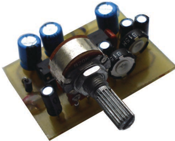
Photo 5: The headphone monitor module is shown without the rotary pickup selector switch.
