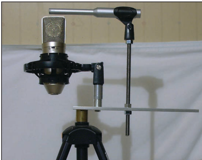
Photo 3: I used a Behringer EMC8000 cardioid for the mid microphone and an Apex 415 set to figure-eight (it has a switch that also enables you to choose omnidirectional or cardioid) for the side microphone in this Mid-Side setup.
