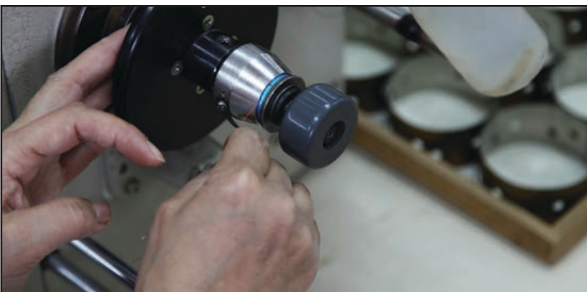
Morel still uses in-house voice coil winding. (Photo courtesy of Morel)
