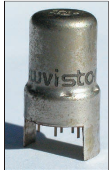
Photo 2: A few low-voltage tubes used nuvistor packages.
