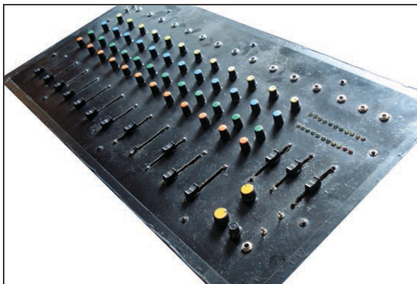
Photo 2. This prototype has 12 inputs and uses three-band tone control modules at each input.
