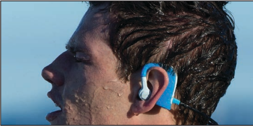
Photo 3: The BlueAnt's Pump HD Sportbuds use sophisticated wind noise suppression. The IP 67 rating means they have excellent resistance to dust, dirt, and water—to the point of being immersible. (Photo courtesy of BlueAnt Wireless)
