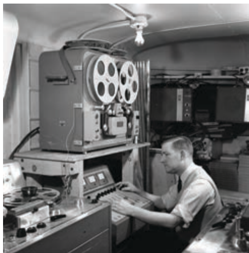
Photo 4: Bob Eberenz adjusts the faders at a Detroit Symphony session in 1962 with the truck outfitted for 35-mm magnetic film recording. (Photo courtesy of Tom Fine/www.preservationsound.com)
