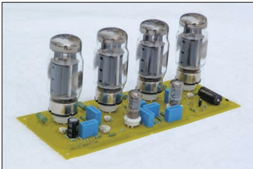
Photo 2: The KT 120 vacuum tubes are big tubes with big electrodes.
