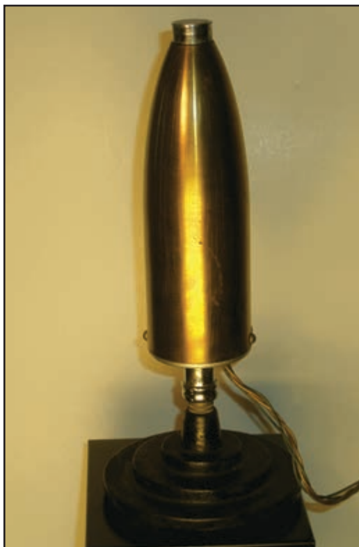
Photo 1: The Western Electric 640AA was the first measurement microphone used at the National Bureau of Standards, which is now known as the National Institute of Standards and Technology (NIST). It is still used by the NIST today.
