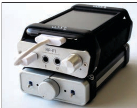
Photo 4: The Fostex HP-P1 portable amplifier and DAC is shown as a “stackup” with an iPhone. (Photo courtesy of Fostex)
