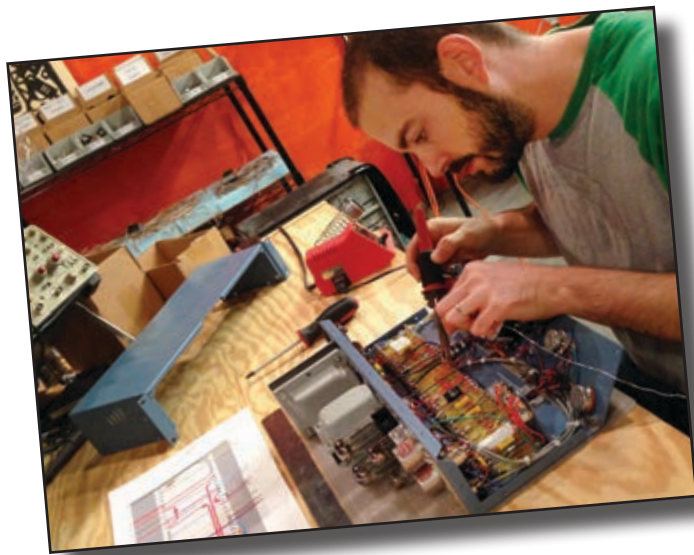
Locomotive Audio founder Eric Strouth hand-builds one of his 14B mono tube compressors.
