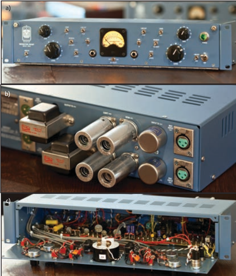
The dual-channel 286A, shown in front (a) and rear (b) views, has a single-ended Class-A tube signal path. Inspired by the vintage Ampex 601 vacuum tube tape recorder, the 286A features two tubes per channel—one EF806 and one 12AY7 (c).
