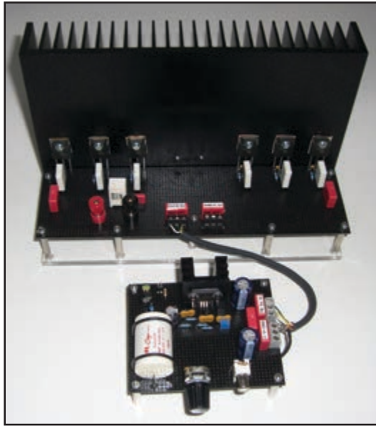
Photo 3: The TERESA amplifier can drive three pairs of transistors.
