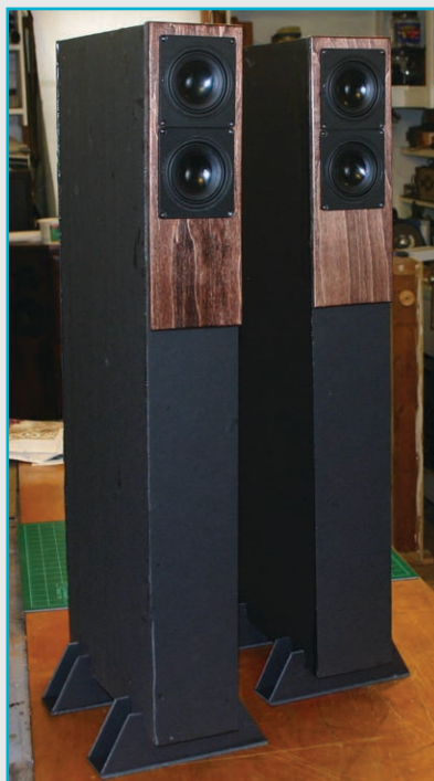
Photo 1: Prototype enclosures can be built from foam board.
