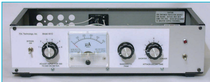
Photo 1: This is the front panel of prototype I built to test the Texas Instruments LM1894 dynamic noise reduction (DNR) system. The panel meter sets the input signal level.
