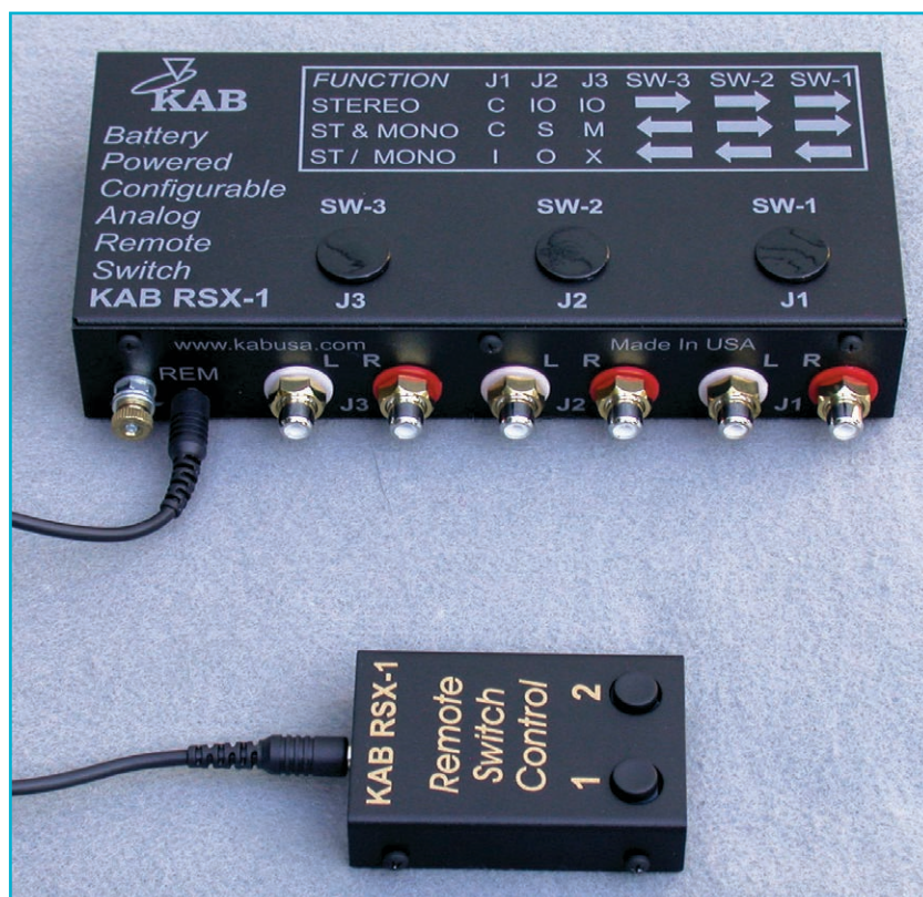
Photo 1: The KAB Electro Acoustics RSX-1 analog remote switch provides clean, noise-free switching for phono and line-level signals. It can also function as a stereo/mono switch.
