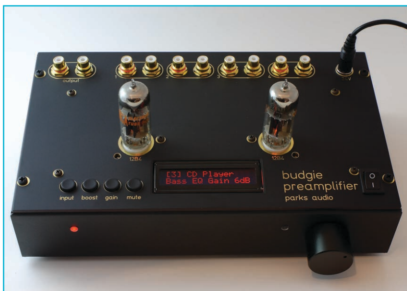
Photo 1: The Budgie preamplifier contains a single-ended, Class-A, all vacuum tube audio path.
