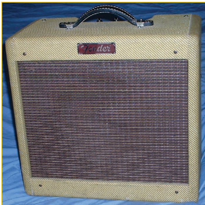
Photo 1: The Fender Pro Junior is a 15-W tube amplifier with a traditional design.
