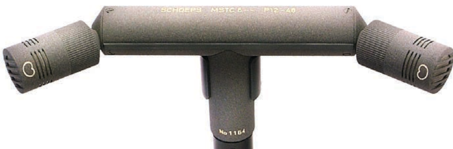
Photo 6: A Schoeps MSTC-64 ORTF stereo microphone is shown. Two MK-4 cardioid capsules are held at a 17-cm spacing and a 110° angle by the MSTC-6 dual amplifier body. (Photo courtesy of Schoeps)
