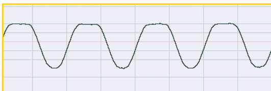
Figure 12: When the preamplifier is overdriven, it produces this output waveform.
