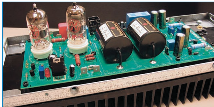
Photo 2: The amplifier design uses a combination of transistors and valves.
