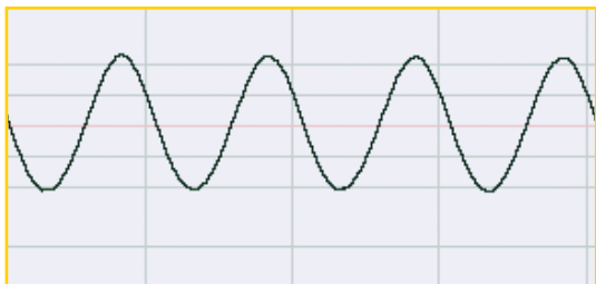
Figure 1: The 35-mV sine wave was fed to the preamplifier.
