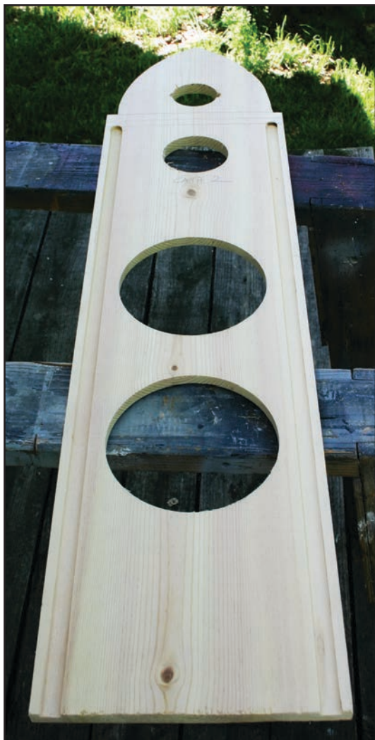
Photo 4: The front panel is shown in detail. Note the dado grooves I made for the side panels.
