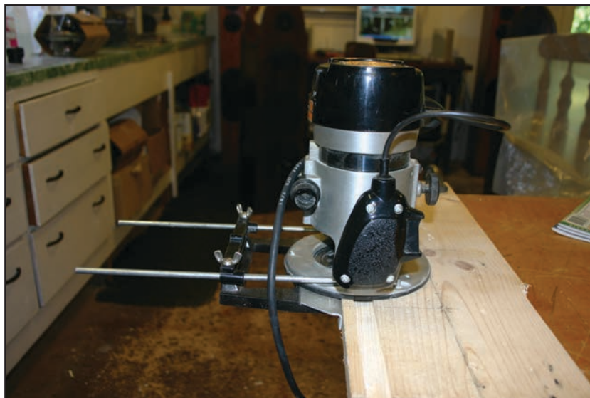
Photo 5: I used a router to make dado grooves in the enclosure.
