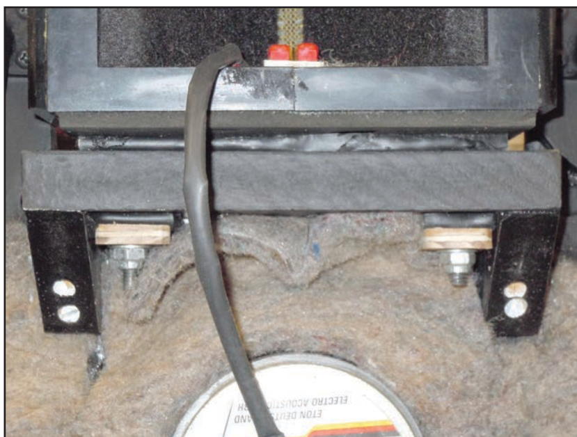
Photo 4: Mount the tweeter on the baffle shelf with layers of Sorbothane between the tweeter and rubber tubing around the bolts. Also use Sorbothane under the bolt mounting plates.
