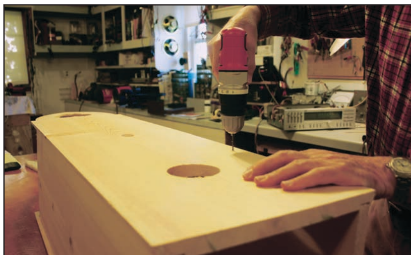
Photo 6: A key component for a polished finish is to drill the starter holes for the finishing nails.
