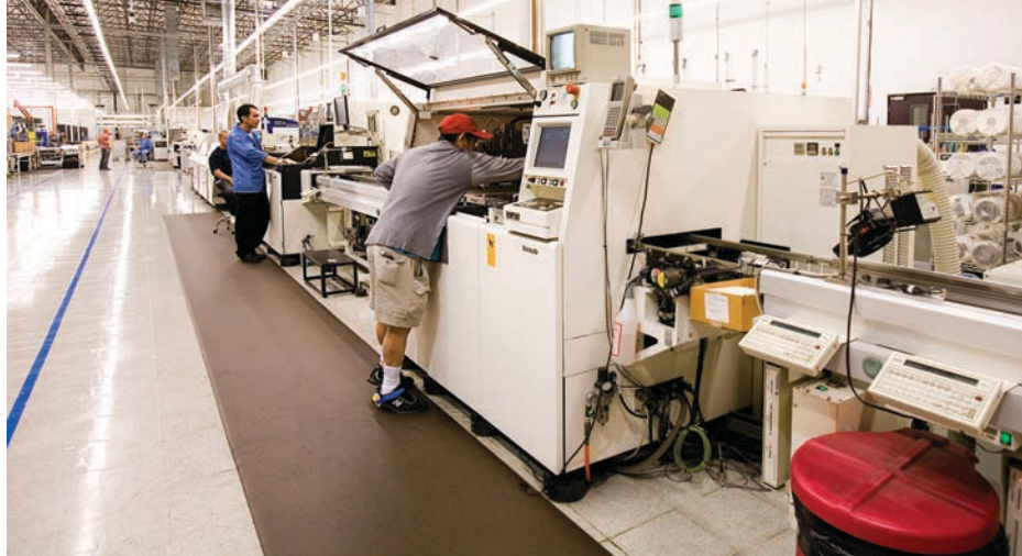
Photo 8: Part of QSC's FAST amplifiers' assembly process includes automated parts placement.
