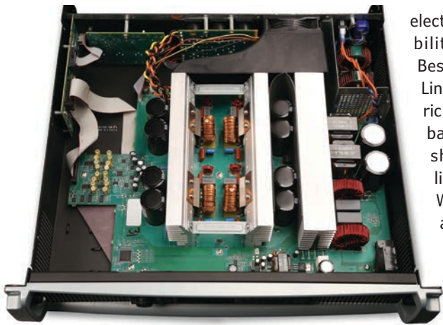
Photo 6: QSC's new amplifier platform was designed as a custom Class-D multichannel high-performance device with agile power distribution across one, two, three, or four channels via Flexible Amplifier Summing Technology (FAST). It also has a PowerLight universal switchmode power supply with power factor correction (PFC) for high efficiency and low weight.
