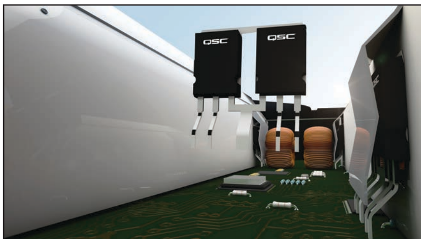
Photo 3: QSC's proprietary output MOSFET packaging contains two MOSFETs (presumably matched at the die phase) and steering circuitry.
