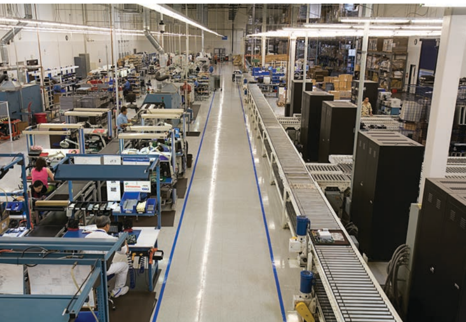
Photo 7: The QSC assembly line in Costa Mesa, CA, is set up in a sequential workflow arrangement to produce a product from start to finish by physically grouping tasks and machines to minimize unnecessary time and motion expenditures.
