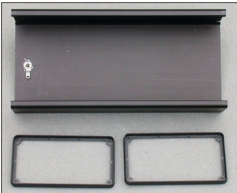
Photo 3: The Hammond 1455-series enclosure's U-shaped body uses a ground lug which, when mated with a slip-on connector from the main chassis, will ensure a proper ground connection. The plastic bezels shown at the bottom are supplied with the enclosure, but their use is optional.
