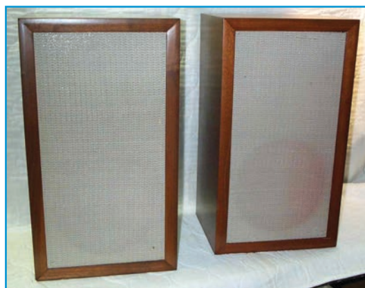
Photo 5: The AR-1Ws are compact sealed enclosures that contain high-excursion woofers.
