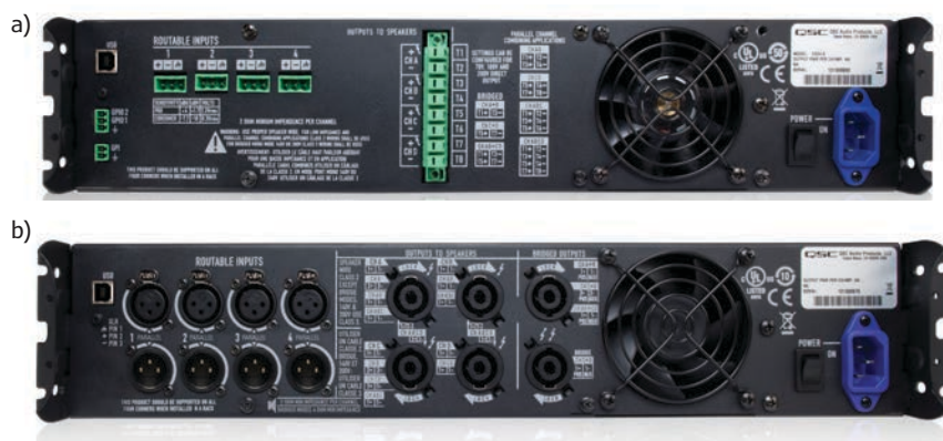
Photo 2: The CXD lineup includes three models. The rear panel features four balanced Euroblock input connectors and four Euroblock touch-proof loudspeaker connectors enabling integrators to terminate wiring before connecting to the amplifier (a). The PLD series, designed specifically for portable sound applications, also consists of three models from 400 to 1,150 W/channel at 8 \Omega (continuous) with four balanced XLR input connectors with loop-thru and six Speakon NL4 loudspeaker connectors for easy setup (b).
