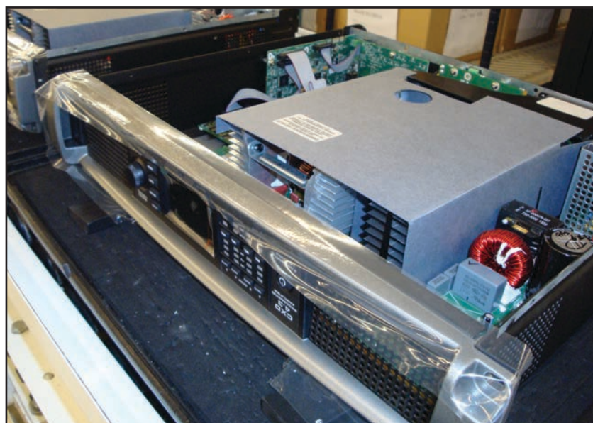
Photo 4: This isn't a top view of the interior; it's a bottom view! Note the inverted construction, which QSC uses to avoid dust collecting on the circuitry and heatsinks.
