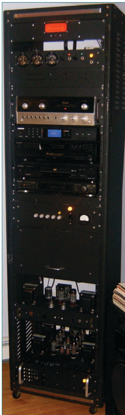
The "Frankenstein" home-theater system used 23 vacuum tubes, powered by 535 VDC of plate voltage over 20 A of filament current, protected by a 10-A main circuit breaker and more than a dozen 3AG fuses.
