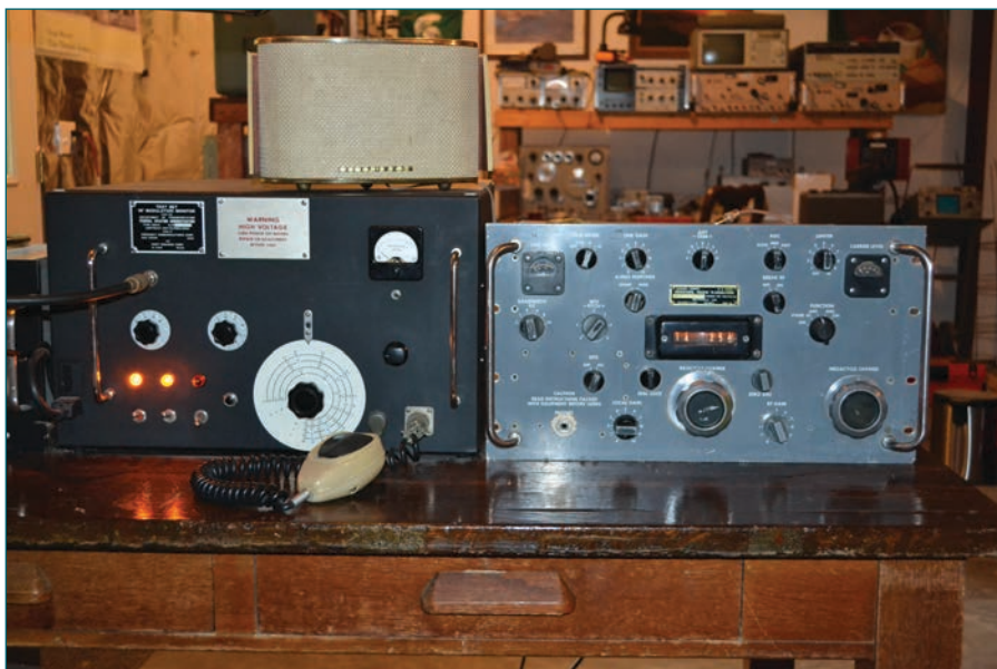
Gregory's go-to vacuum-tube transceiver is a 20-m single-sideband (SSB) of his own design.
