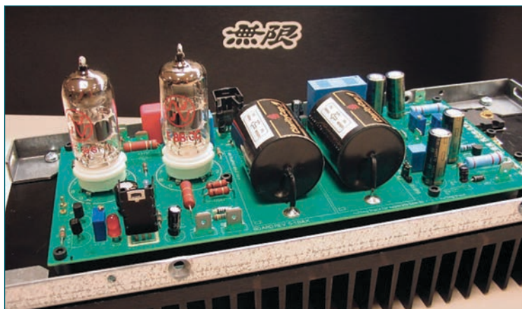
Photo 2: The amplifier uses a mixture of transistors and valves.
