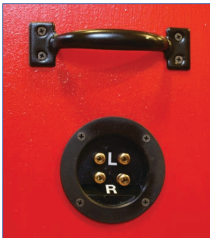
Photo 7: I added banana jacks to a single-speaker cup to accommodate both channels. The optional handle makes moving the tower easier.
