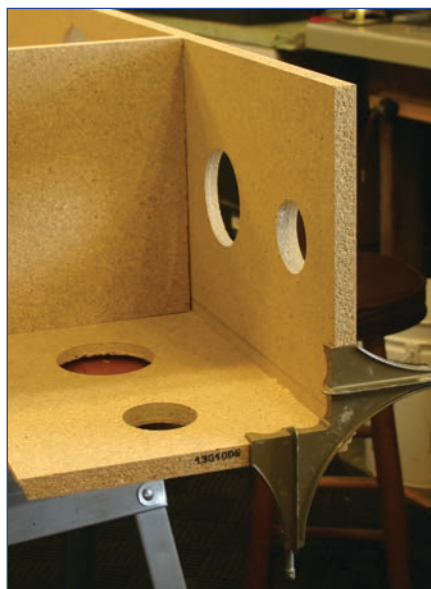
Photo 5: Simple butt joints were used in the assembly, along with glue and 2" finishing nails.
