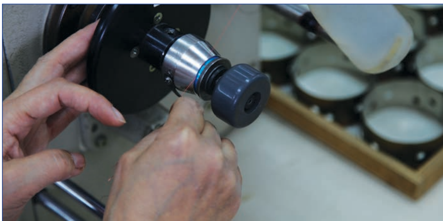
In-house voice coil winding has been a fundamental element for Morel. Here, a Morel employee winds aluminum wire on an aluminum bobbin (former) to manufacture a tweeter voice coil. (Photo courtesy of Morel)
