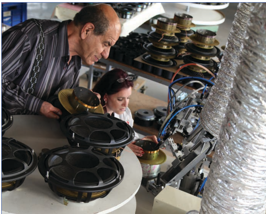
A glimpse into a soon-to-be released driver. Meir Mordechai meticulously inspects his latest development—a titanium-based subwoofer (which is a new addition to the Ti driver series) during its cone-assembly process. (Photo courtesy of Morel)
