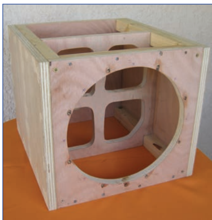
Photo 1: The subwoofer box's interior is shown in the early phases of construction.
