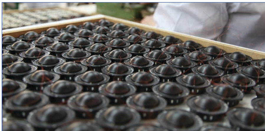
A tray of soft dome tweeters works its way through the manufacturing line at Morel's factory in Israel. (Photo courtesy of Morel)
