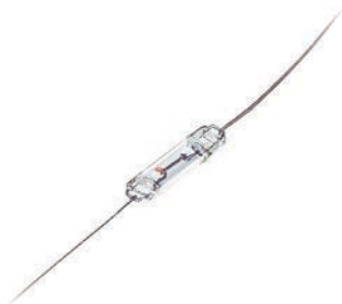
Photo 3: Loudspeaker protection light bulbs are sometimes used in high-output speaker products. (Photo courtesy of JBL)
