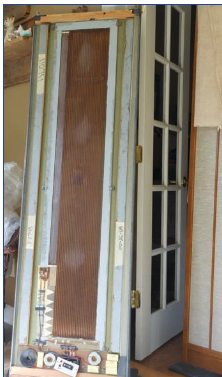
Photo 2: The Maggie's backside is shown without the obscuring grille. A stretched 10" x 56" polyester diaphragm on a 24" x 70" baffle is visible. The woofer section is 8" x 56" (note the heavy wire). The treble section is 1.5" x 45". The magnet structure is on the frontside, and not visible here. Maggies are inherently "single-ended."
