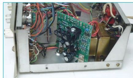
Updatemydynaco now makes a regulated power supply upgrade kit for the PAT-4 preamplifier.
