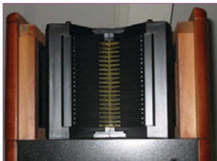
Photo 1: Unlike a normal piston loudspeaker, the ESS Air Motion Transformer linearly squeezes and expands its diaphragm.
