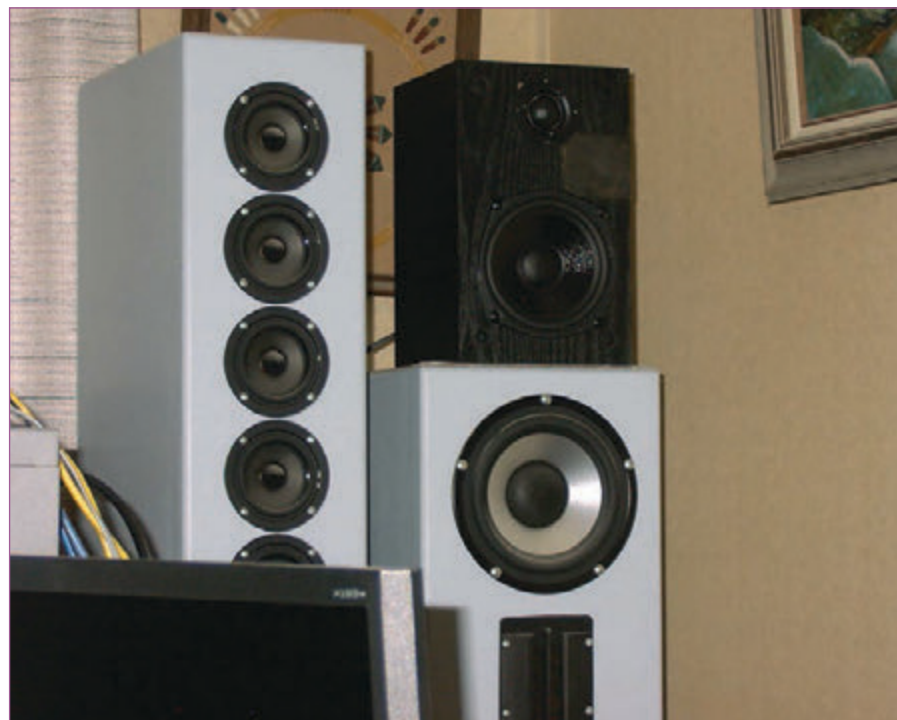
Photo 4: This listening test setup includes a partial view of one of the nine-driver line arrays. The right and left speakers are about 18' apart.
