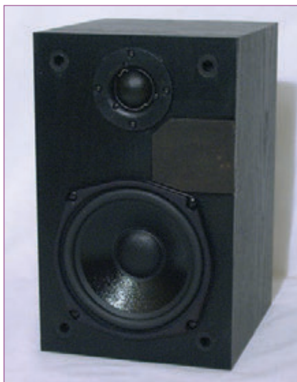
Photo 3: This is the completely rebuilt MTX 5i, showing the new drivers and the patch covering the vent hole.
