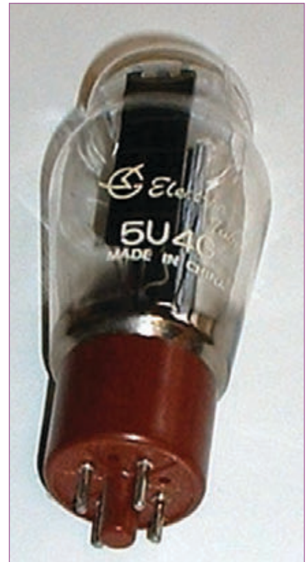
Photo 1: The 5U4G family includes some of the most popular octal full-wave rectifiers.
