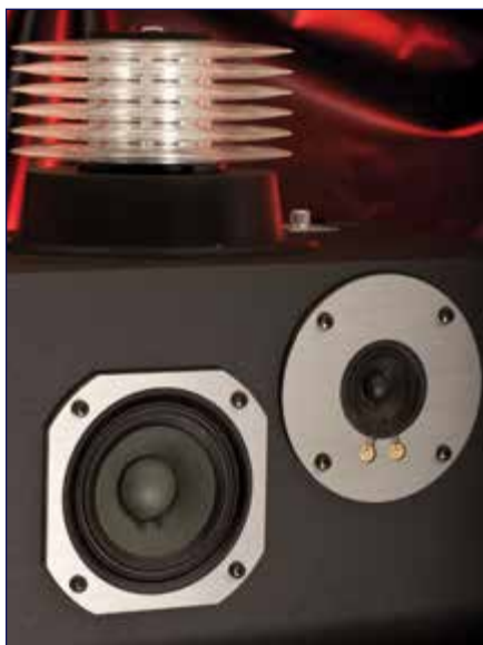
Photo 2: The Pioneer HPM 150 tweeter, released in the late 1970s, used a new version of the PVDF tweeter, but it retained its omnidirectional characteristics.
