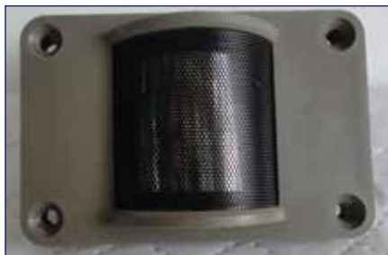
Photo 1: Pioneer's HPM-100 tweeter was among the few technically successful efforts involving high-polymer film transducers.
