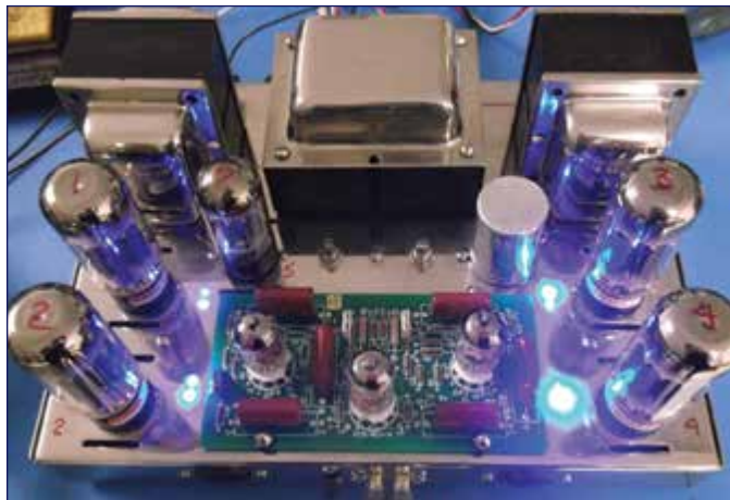
Photo 10: The alternate project calls for balanced potentiometers installed on a new driver board.
