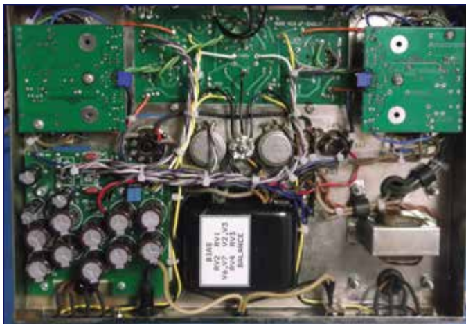
Photo 11: An alternate project shows trim potentiometers added to the two comparator boards.
