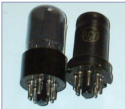
Photo 4: These two 12SN7 dual triodes have octal envelopes. One is glass. The other is metal.
