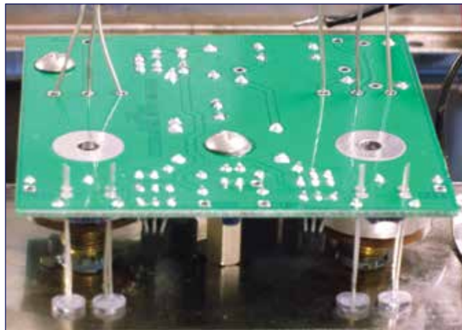
Photo 6: The LEDs are positioned in place.
