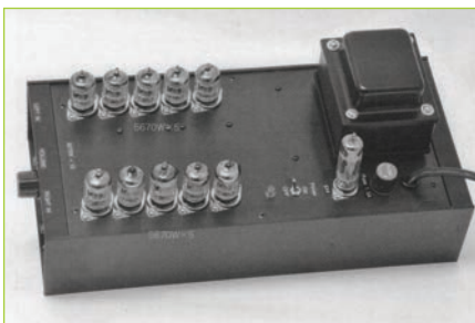
Photo 2: The four-parallel push-pull amplifier is shown from the side.
