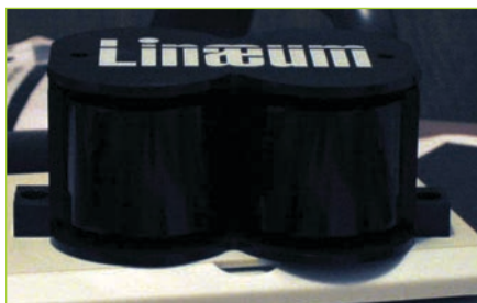
Photo 2: The Linaeum tweeter has a voice coil, which is flattened into a vertical shape and suspended between opposing rectangular magnet poles. (Photo courtesy of Linaeum)
