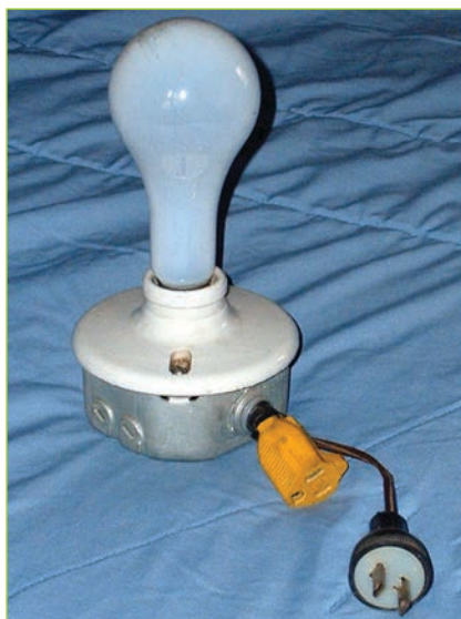
Photo 1: The test fixture connects an incandescent light bulb in series with the equipment being tested. If the bulb lights, something is drawing too much current.
