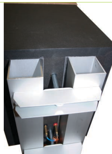
Photo 2: Once complete, the enclosures are attached to the aluminum guidance bearings.
