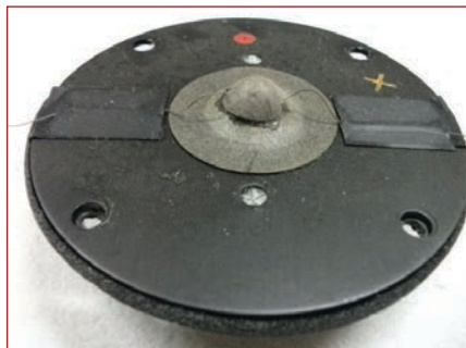
Photo 3: The Allison tweeter has a larger diaphragm with a small effective radiating area.
