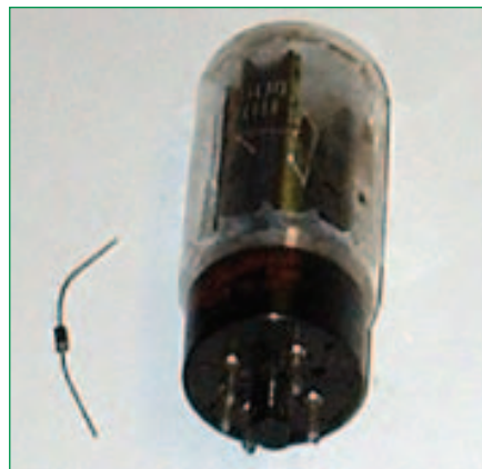
Photo 2: The solid-state diode (left) is dwarfed by the 5U4GB hollow-state diode (right).
