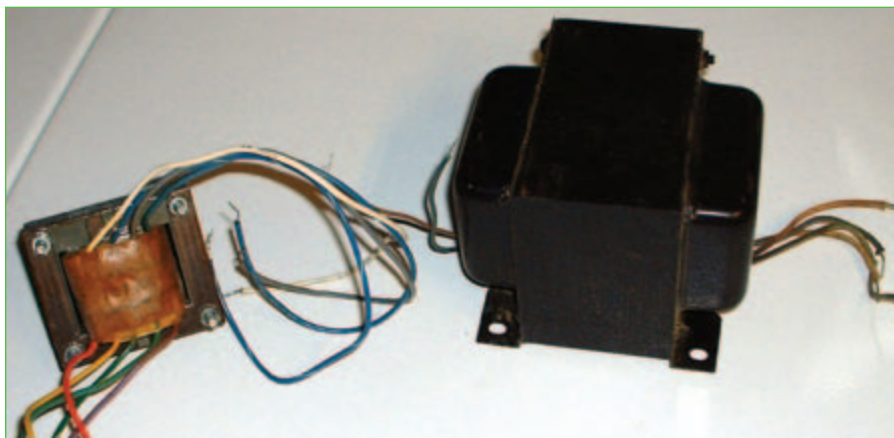
Photo 1: Power transformers vary in size. Some large ones have steel case enclosures.
