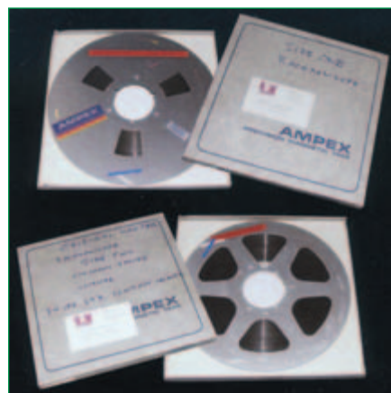
Photo 3: David Hancock's original 30-ips tapes—two 14" reels—were used for Analogue Productions's latest remasterings of Symphonic Dances . "Constant velocity" refers to the equalization curve used on his custom-modified "Plywood Ampex" tape recorder. Ampex 456 tape didn't exist in 1967, so Hancock must have spun the first tape onto a new reel and stored both in new boxes, at some point. (Photo included with the SACD edition, reproduced courtesy of Analogue Productions)
