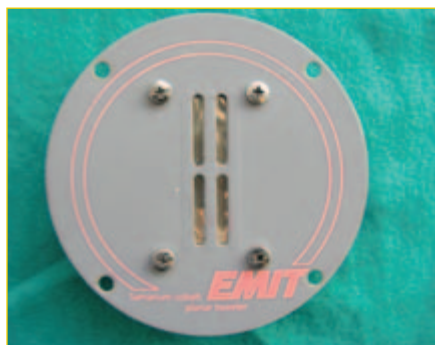
Photo 4: Infinity’s EMIT tweeter used powerful Samarium cobalt magnets covered by a thin mylar polyester diaphragm.
