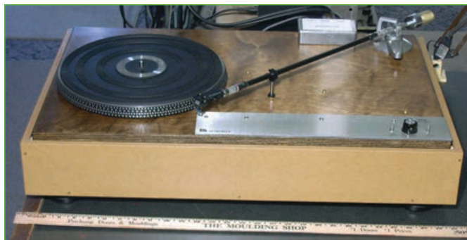
Photo 1: This is the completed second Netronics 350D rebuild. The only remaining original parts are the direct-drive DC motor, the platter, the aluminum nameplate with switches, and the 33-1/3 and 45 RPM speed control.
