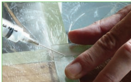
Photo 4: Use acrylic adhesive to tack the plastic spacers together.
