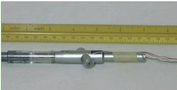
Photo 3: Epoxy connects the gimbal tube to the carbon fiber tube with a 1.5"-long acrylic collar. Masking tape is used to hold the small gauge solder wires that go through the gimbal.
