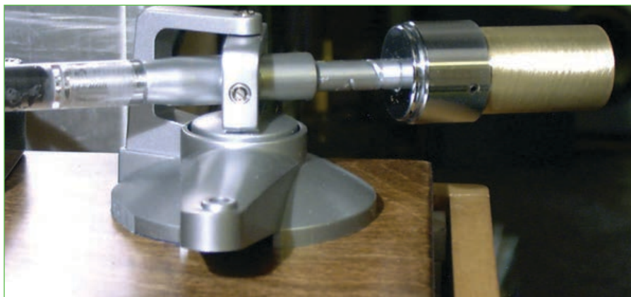
Photo 8: The gimbal salvaged from the Stanton turntable was rebuilt with a heavier counterweight. The added weight slides into the rear of the original weight and is secured by two set screws. The original calibrated dial was removed because it's not accurate with the weight increase. A gauge must be used to set the stylus force.
