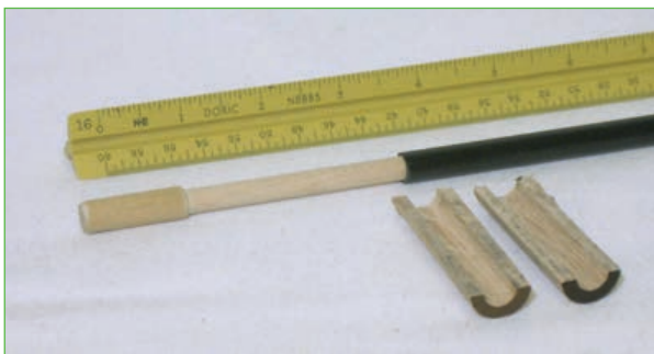
Photo 2: These are key carbon-fiber tube machining aids. The split hardwood tube, about 2.5" long, spreads the pressure on the tube circumference when held in the lathe chuck. The inside wooden rod stabilizes the tube for cutting.
