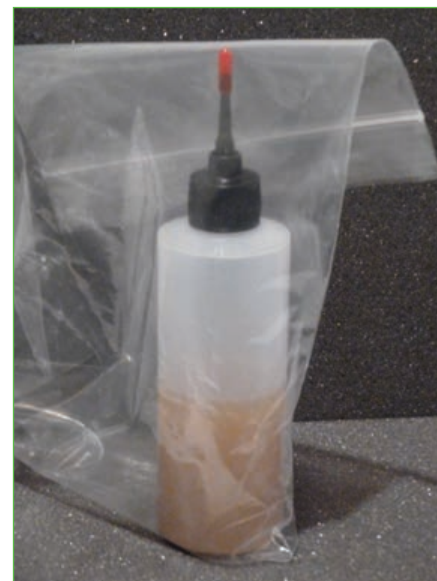
Photo 3: A plastic bottle and needle from Howard Electronics is used to apply the ER Audio polyurethane.
