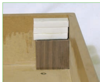
Photo 5: One corner of the base unit with a wooden block and stack of three art gum erasers was used to support the motor board. Rubber cement was used to lightly connect the erasers. The small circle in front of the block is an embedded nut the foot screws into.
