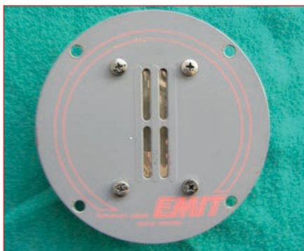
Photo 3: EMIT Tweeter Planar film diaphragm printed circuit tweeters often used SmCo magnets for enhanced performance.
