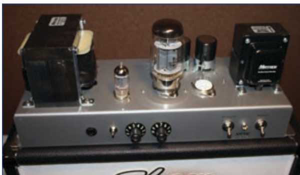
Photo 3: Shaw Audio Tonerod SE chassis. Note the large output transformer at left for the Class A 6550 output tube (Source: Shaw Audio)
