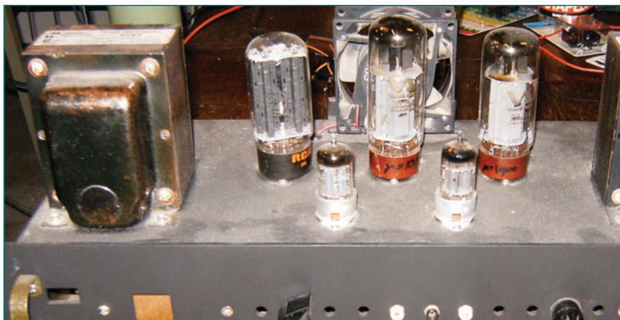
Photo 2: A mono-block power amplifier
