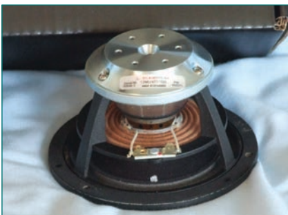
Photo 2: The 12MU is built with a neodymium ring magnet motor structure.
