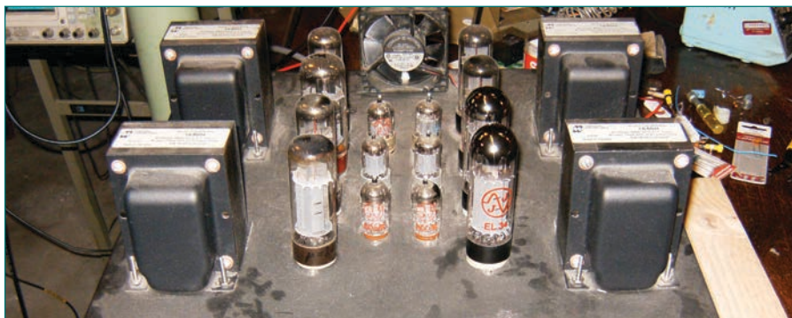
Photo 5: A mono-block power amplifier
