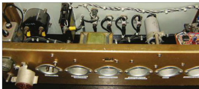
Photo 7: An inside view of the rear of the power distribution showing front-panel fuses
