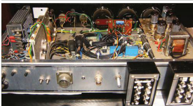
Photo 4: A rear view of the transfer switch and surround pre-amplifier showing rear-panel audio input and output connections
