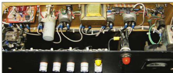
Photo 6: Inside the front of the power distribution, showing 120-VAC outlets and relay driver
