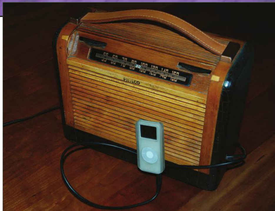
Photo 1: A 1948 Philco portable tube radio restored and repurposed as an MP3 amplifier
