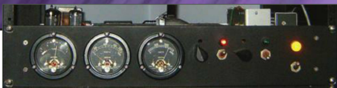
Photo 2: The transfer switch and surround pre-amplifier
