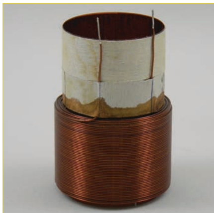
Photo 6: A voice coil with a Nomex bobbin (Source: Precision Econowind)
