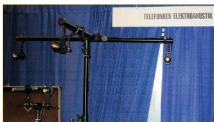
Photo 3: Telefunken Elektroakustik's ELA M260 Tri-Mono recording system, recreated the classic Decca Tree introduced for stereophonic orchestra recording in the mid-1950s. In the lower left, the same microphones are shown on a small bracket suitable for coincident stereo recording or a near-coincident ORTF configuration.
