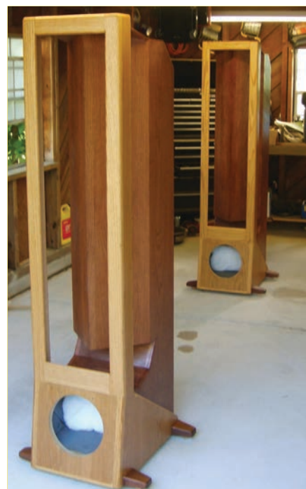
Photo 2: The “beam-splitter” cabinets are ready for the woofers and stat-panels. The angled box faces behind the panel opening to form the “beam-splitter.”
