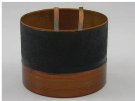
Photo 7: A voice coil with a composite bobbin (Source: Precision Econowind)
