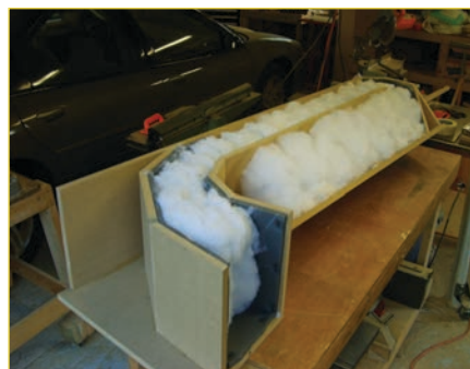
Photo 3: The transmission-line cabinet, partially complete with fiber stuffing in place.
