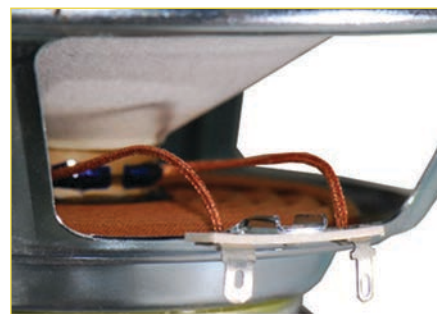
Photo 2: Lead wires attached at speaker terminals (Source: Taiwan Maiden)
