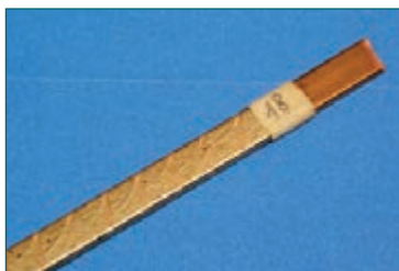
Photo 8: A close-up view of an aluminum flat wire (Source: HM Wire International)
