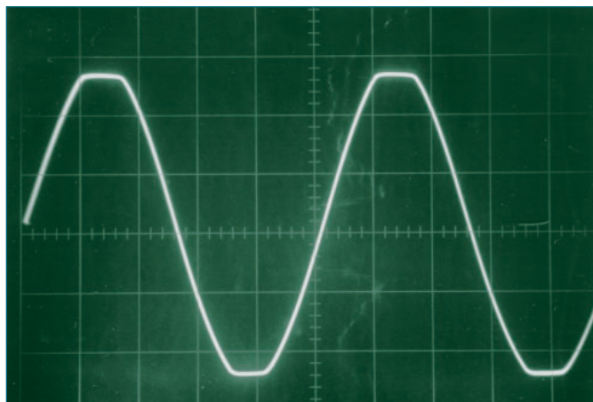
Photo 4: The clipping behavior at 11 W/1 kHz (5 V/div)
