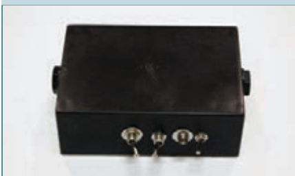
DIY MPF102 High-Impedance Preamplifier (also known as the piezo preamplifier): "This is another high-impedance preamplifier we designed with a JFET, and the sound is loud and clean—can't ask for much more than that!"
