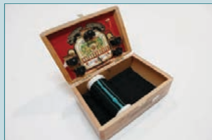
DIY Foxhole Radio AM Receiver/Germanium Diode Crystal Radio: "Soldiers in WWII used to make these radios with items they found in their foxholes. They can receive AM transmissions with surprising clarity and the radios don't require battery power!"
