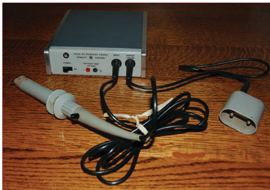
Photo 1: An HP 456A fresh from a surplus electronic equipment store. Note the lack of a power cord (indicating that it contains batteries) and the covered banana plug output connector.
