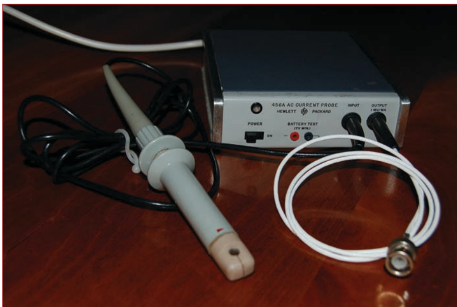
Photo 9: BNC output cable installed
