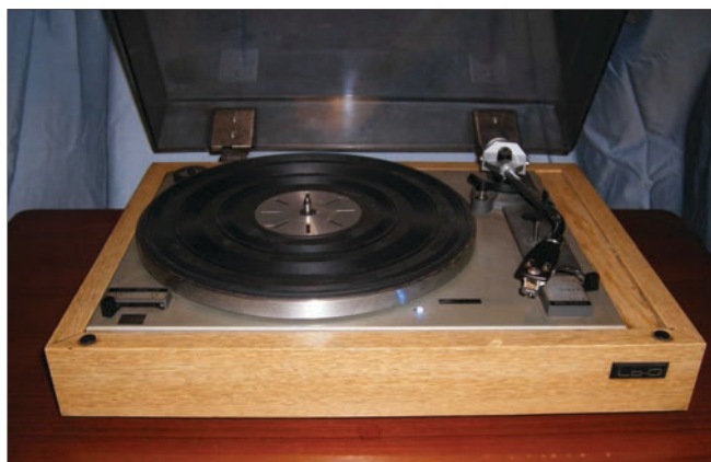
Photo 1: This is a front view of a modified turntable. The blue LED indicates that the player system is on.
