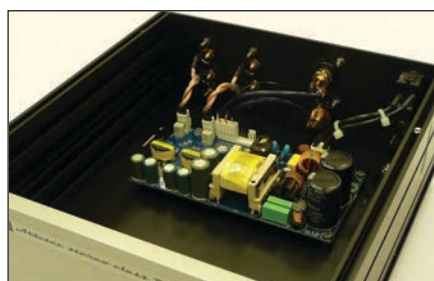
Photo 4c: Inside overview Abletec class D amplifier
