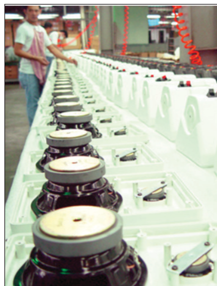
Photo 6: Speakers on a semi-automatic production line in the Philippines. (Photo courtesy of Dai-Ichi Electronics)
