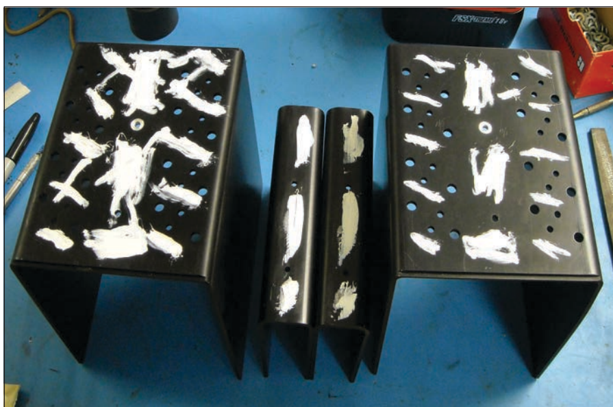
Photo 5: Grease applied to heatsinks
