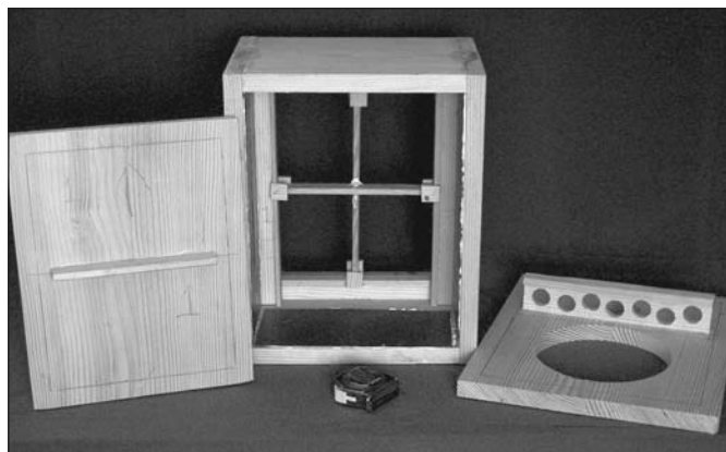
PHOTO 2: Cabinet components before assembly.
