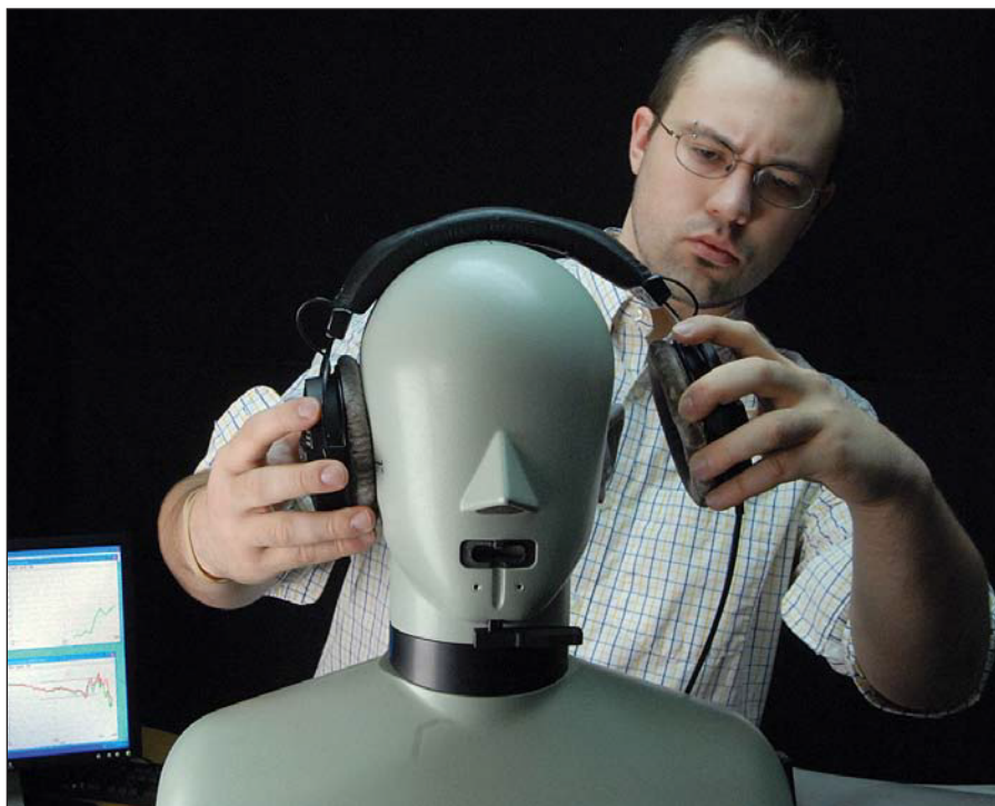
FIGURE 9: Mark Brezinski, editor-in-chief of Headphoneinfo.com, part of the Reviewed.com family of product review websites, uses the setup described here with a head and torso simulator to carry out objective measurements of the audio quality of many different brands of headphones. The audio test forms part of a complete battery of tests which also examine noise cancellation and sound leakage. They also conduct additional tests that provide readers information on the comfort, usability, and design of headphones (credit Richard Baguley/Reviewed.com).
