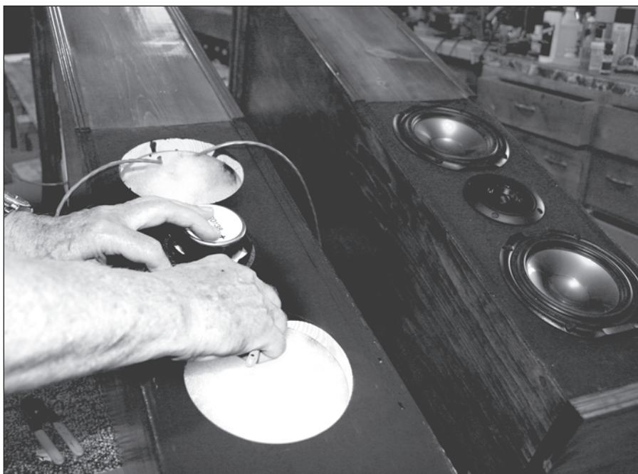
PHOTO 7: Wiring mids and tweeter.
