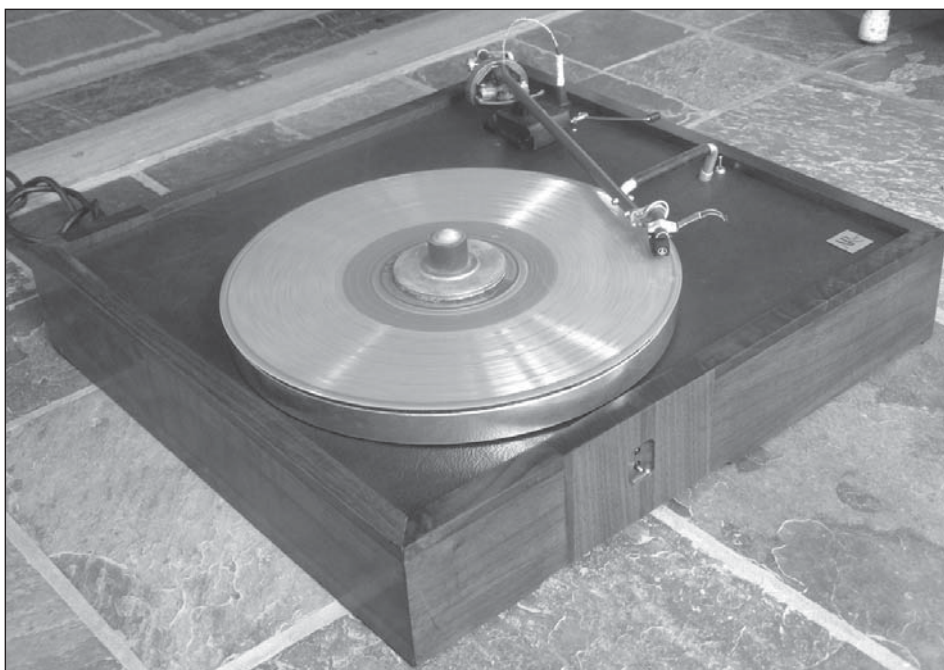
PHOTO 1: An overall perspective shot of the completed table and Defarge arm. The woodwork, leather surfaced motorboard, and scale (approximately 18" × 18") are evident.
