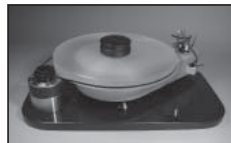
PHOTO 8: Stroboscope "bumps" cast on the platter rim are useful at 33 \frac{1}{3} and 45 RPM only. If the turntable plays 78s, you will need a way to measure the speed.
