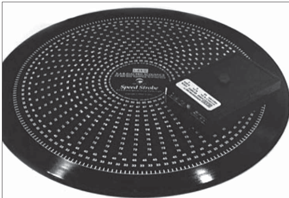
PHOTO 2: The KAB SpeedStrobe™. Instead of bars, this disc has the rotational speed numbers printed on it. The 60Hz light source limits its use to 60Hz powered turntables.
