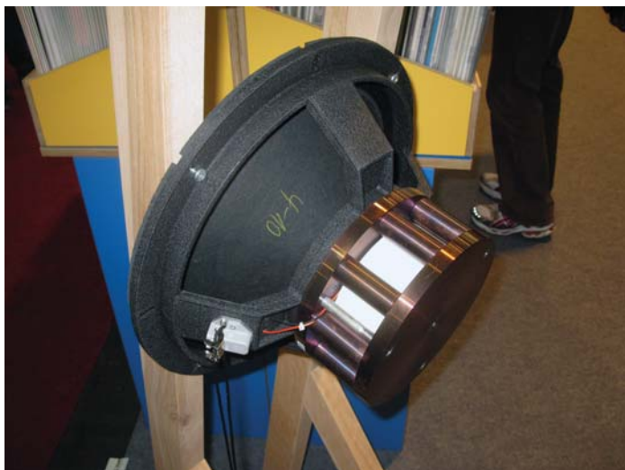
PHOTO 3: The Kilimanjaro-series field coil speaker.
