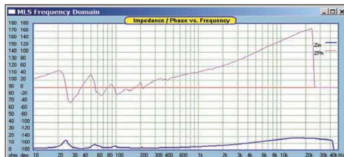
FIGURE 12: The impedance response of a pair of cabinets set up as in Fig. 11. The oversized rear chamber and the 25Hz driver resonance appears to load quite well from the flatter impedance magnitude.
