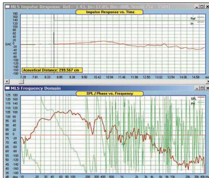
FIGURE 11: The impulse response (top plot), frequency, and phase response (bottom plot) of two cabinets measured outdoors, on the ground and side by side. From 47Hz to 150Hz, the response is flat with the exception of a +3dB hump at 98Hz. Below 47Hz a -6dB shelf is in effect down to 25Hz. Below 25Hz the response rolls off at 24dB per octave.
