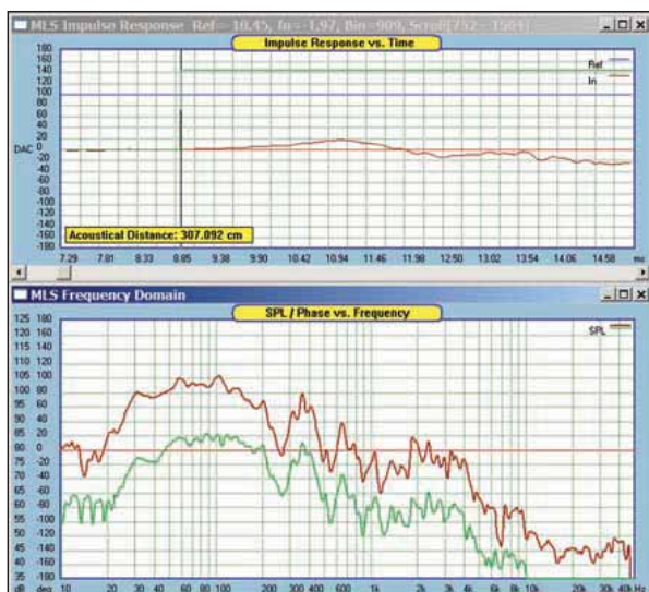
FIGURE 16: Rear volume is reduced to 4ft 3 . Impulse response is shown in the top plot. Bottom plots are wall position frequency (top line) and ground position frequency response shifted -20dB (bottom line) of two cabinets.
