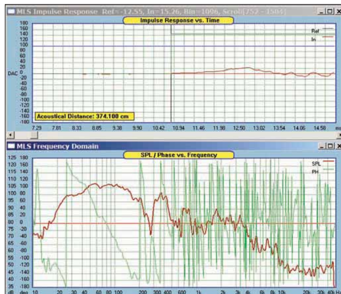
FIGURE 13: The impulse response (top plot), frequency, and phase response (bottom plot) of two cabinets measured outdoors, back against a wall and side by side. Below 45Hz the bottom end is a -5dB shelf down to 25Hz, then the response rolls off at 24dB per octave.
