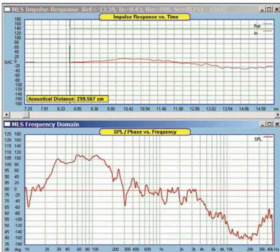
FIGURE 4: Two cabinets placed against a wall, outdoors, measured impulse (top plot) and frequency (bottom plot) response.
