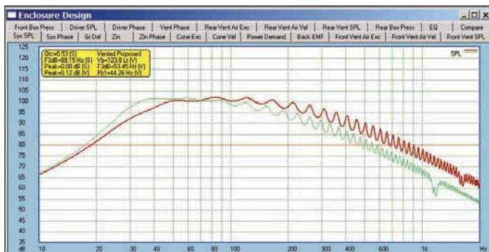
FIGURE 8: SoundEasy simulation of a 30Hz hyperbolic horn. At 30Hz the bottom line is the eighth space size horn simulation. The top line is half space size horn and has greater low-frequency output down to 30Hz.
