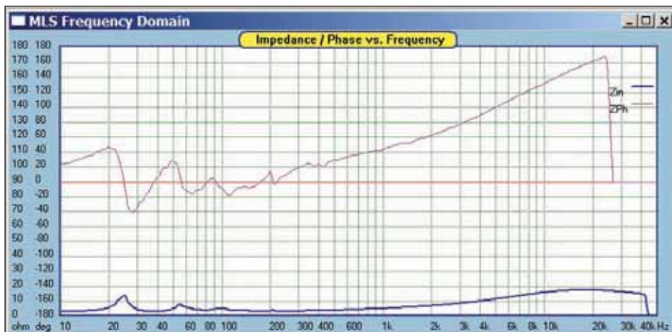
FIGURE 14: Impedance response of the measurement setup of Fig. 13. The wall position provides improved horn loading. All improvements are above 40Hz, where the impedance phase approaches zero.
