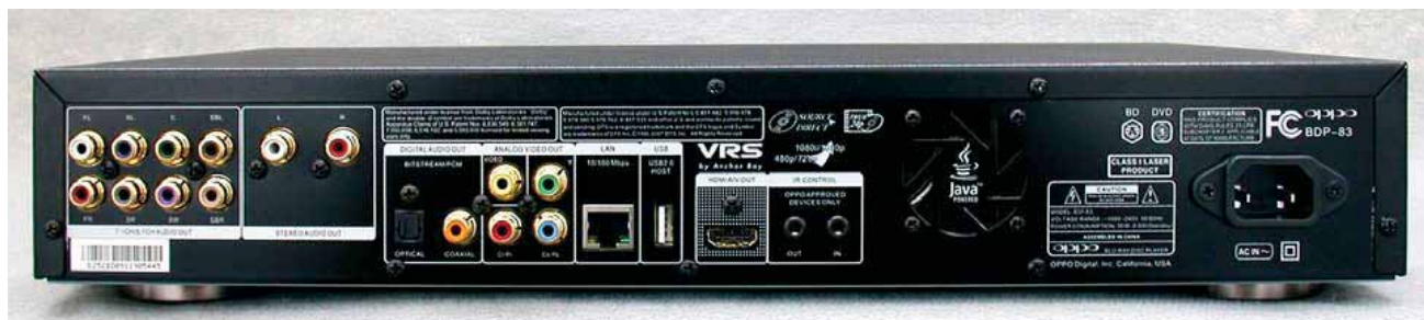
PHOTO 4: Rear view of the BDP-83 player. Analog connections include eight RCA jacks for 7.1-channel surround and two for stereo. The unit also has optical and coax digital outputs, HDMI, component and NTSC composite video connectors, plus a Cat-5E LAN connector.
