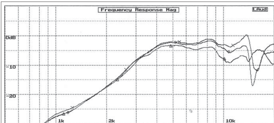
FIGURE 18: On- and off-axis response of tweeter portion of #214 driver.
