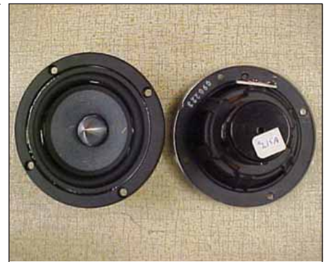
PHOTO 6: Front and rear views of #215 3" mid/tweeter.
