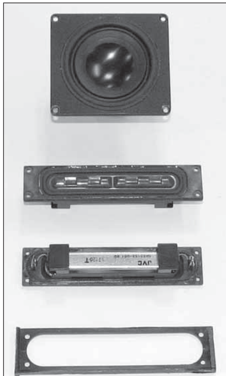
PHOTO 1: The A3 woofer (top) with the 1" × 4" JVC drivers (center). The template (bottom) is used to draw the speaker cutouts.
