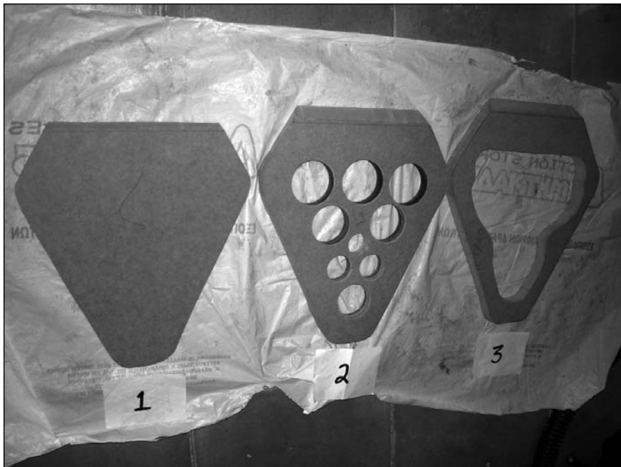
PHOTO 11: First three layers of midrange section. Note perforations in board # 2.
