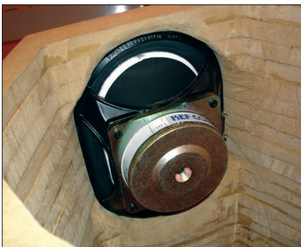
PHOTO 6: Positioning the woofer driver.
