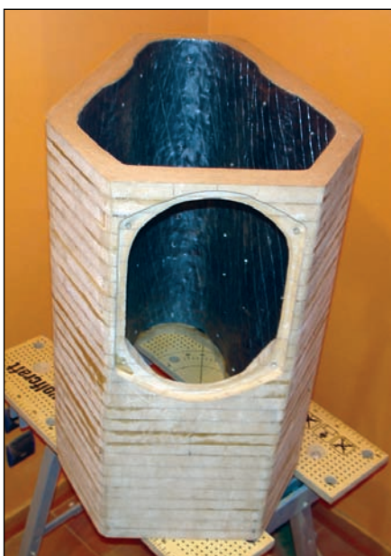
PHOTO 4: The woofer box with sheet of lead installed.
