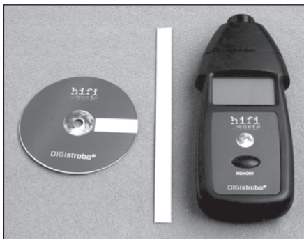
PHOTO 1: HIFI4Music's DIGIS trobo, distributed in the US by Ultra Systems. The device measures turntable speed by reading the reflection off a piece of reflective tape once per revolution. Unfortunately, the readout has only 0.1-rpm resolution, making precise reading of common speeds like 33.33 and 78.26-rpm impossible.
