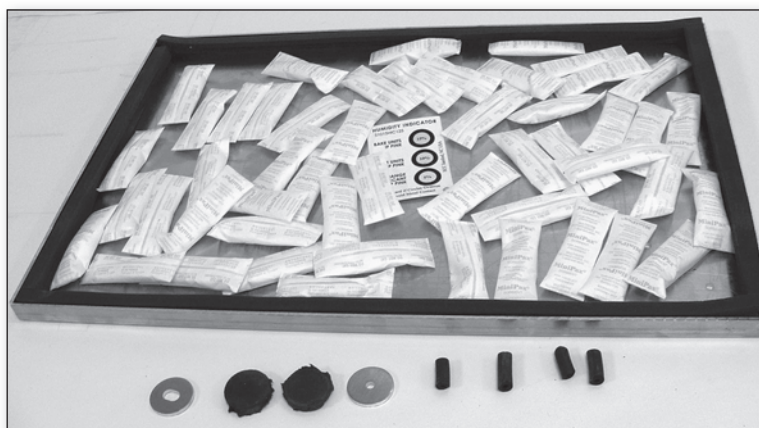
PHOTO 3: Bottom pan with gasket and silica gel, foot parts, and rubber tubing spacers.
