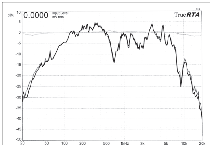
FIGURE 3: Reference and model 818 microphone data shown with the difference curve. TrueRTA using QuickSweep. Half-octave smoothing was applied to the difference data.
