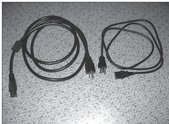
PHOTO 12: Power cords—14 gauge vs. 18 gauge stock.
